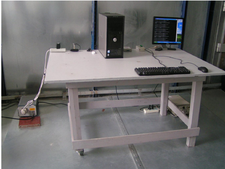
Conducted Emission Test Set-up - Front View
