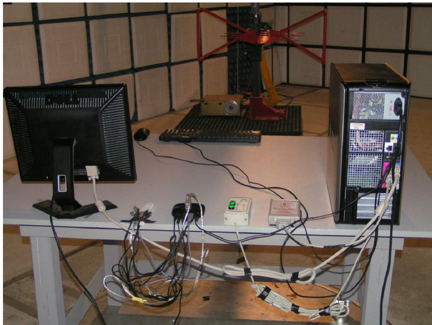
Radiated Emission Low Frequency Test Set-Up – Back View
