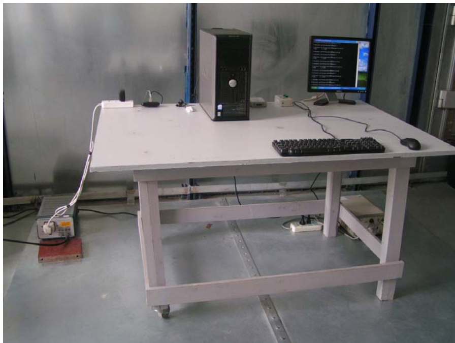
Conducted Emission Test Set-up – Front View
