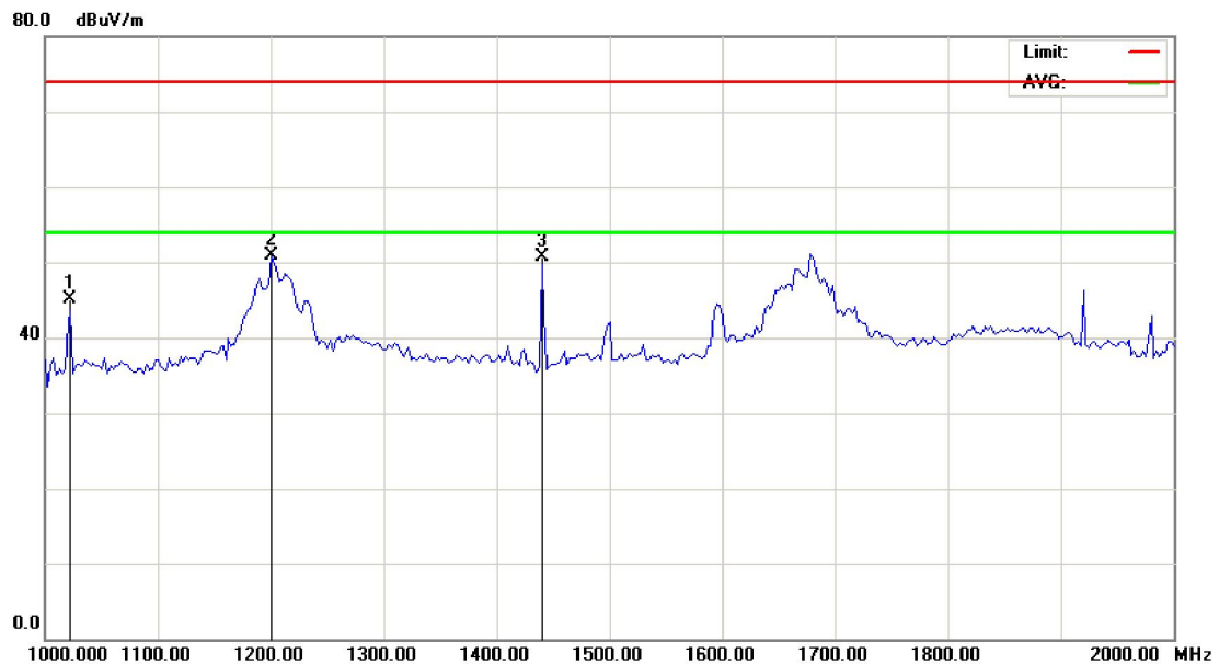
Vertical Radiated Emission Plot (Peak, Max Hold Mode)
