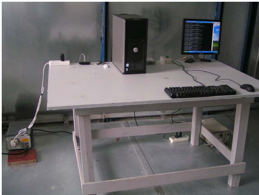
Conducted Emission Test Set-up – Front View
