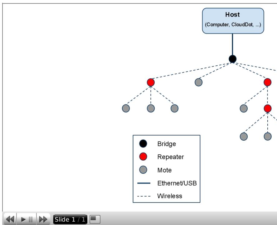
**Bridge:** A bridge is used to connect the wireless network to a host via Ethernet or USB. Each network has only 1 bridge. The wireless transceiver on a bridge is always on. A bridge can have up to 16 children (repeaters and motes).
