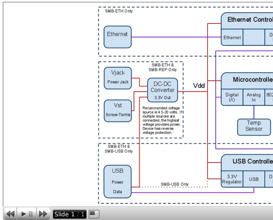
There are 3 ways to provide power to the SMB. Multiple can be connected at the same time, in which case the one with the highest voltage will actually provide power.
