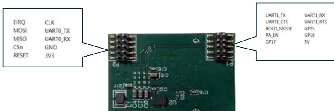
**Warning: The pin header is fragile, please insert the socket carefully.**
