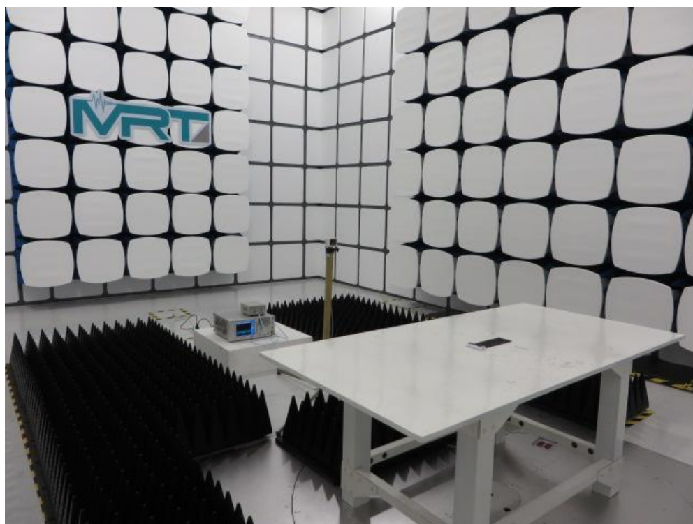
Description: Radiated Emission Test Setup for 18GHz ~ 26.5GHz
