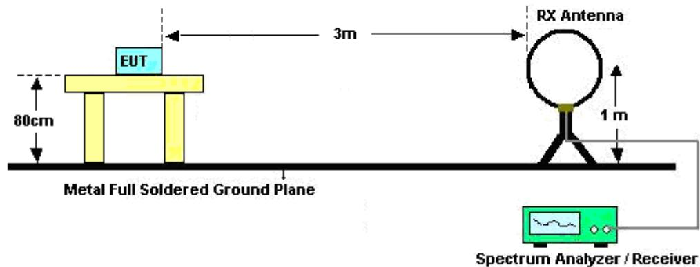
For radiated emissions from 30MHz to 1GHz
