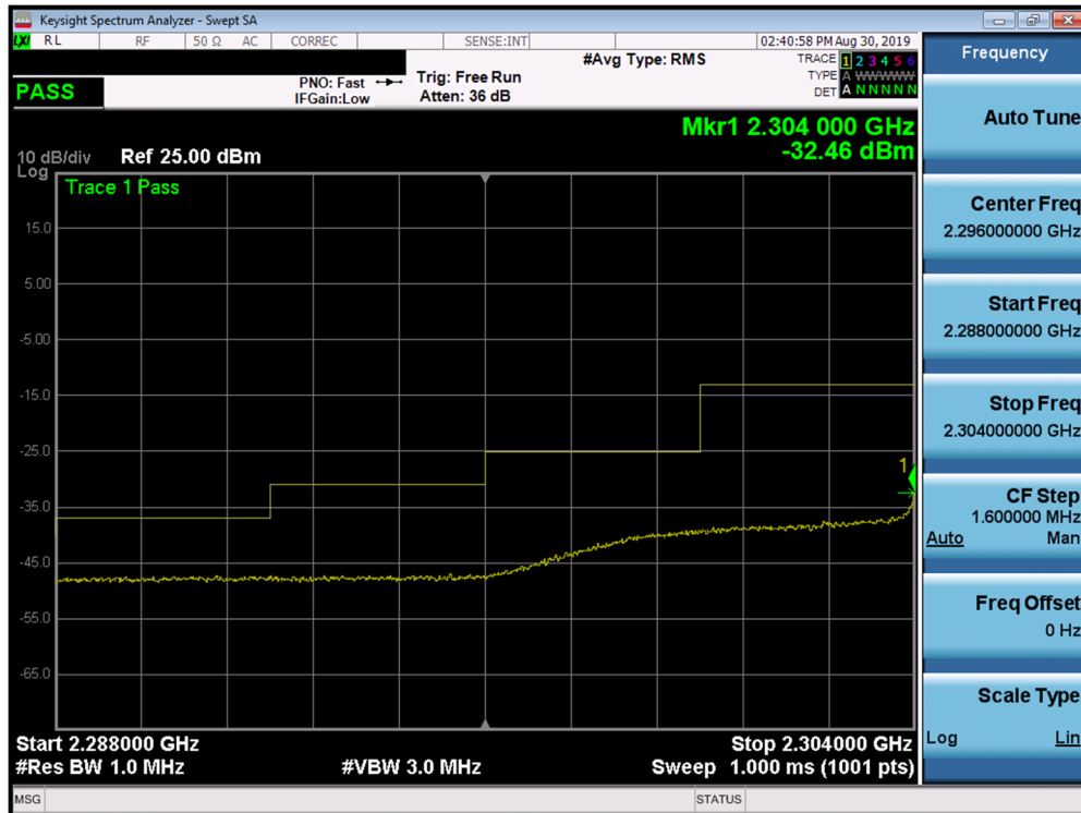
Plot 7-24. Lower Extended Band Edge Plot (Band 30 - 10.0MHz QPSK - Full RB Configuration)
