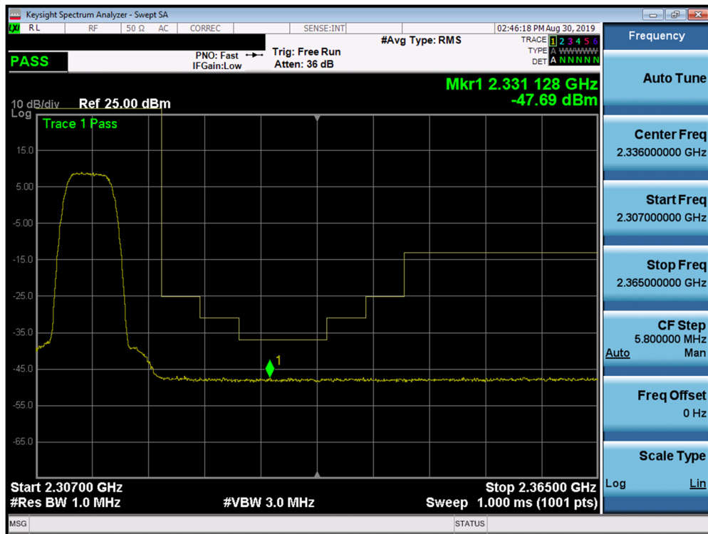
Plot 7-22. Upper Extended Band Edge Plot (Band 30 - 5.0MHz QPSK - Full RB Configuration)
