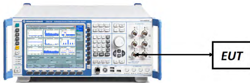
Figure 7-7. ERP/EIRP Measurement Setup
