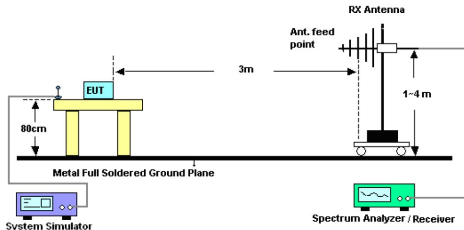
For radiated test above 1GHz
