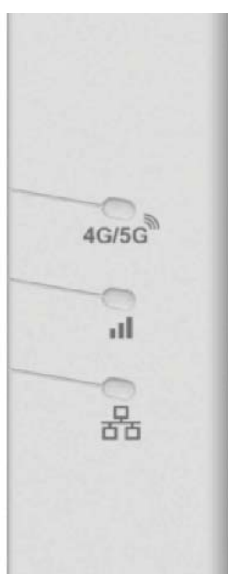
Figure 5 – CFW-2211/3212 LED indicator lights
