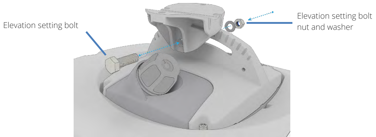
Figure 8 - Attaching the mounting bracket to the AurusPRO 5G Outdoor CPE
