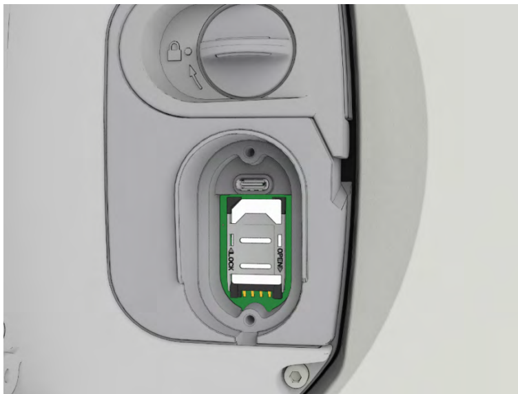
Figure 5 – SIM card locked in place
