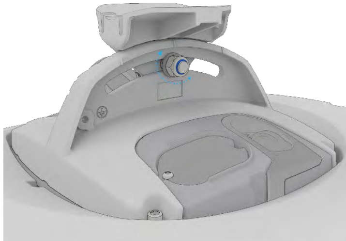
Figure 9 - Assembling mast bracket to mast
