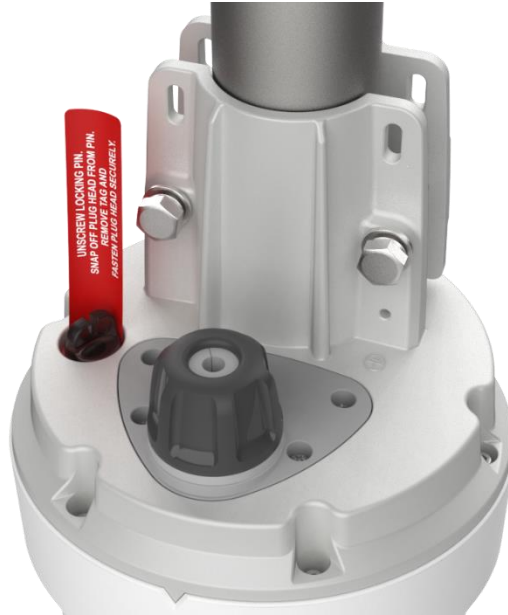
Figure 8 - Ethernet / SIM card cover re-assembled
