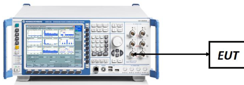
Figure 7-7. ERP/EIRP Measurement Setup
