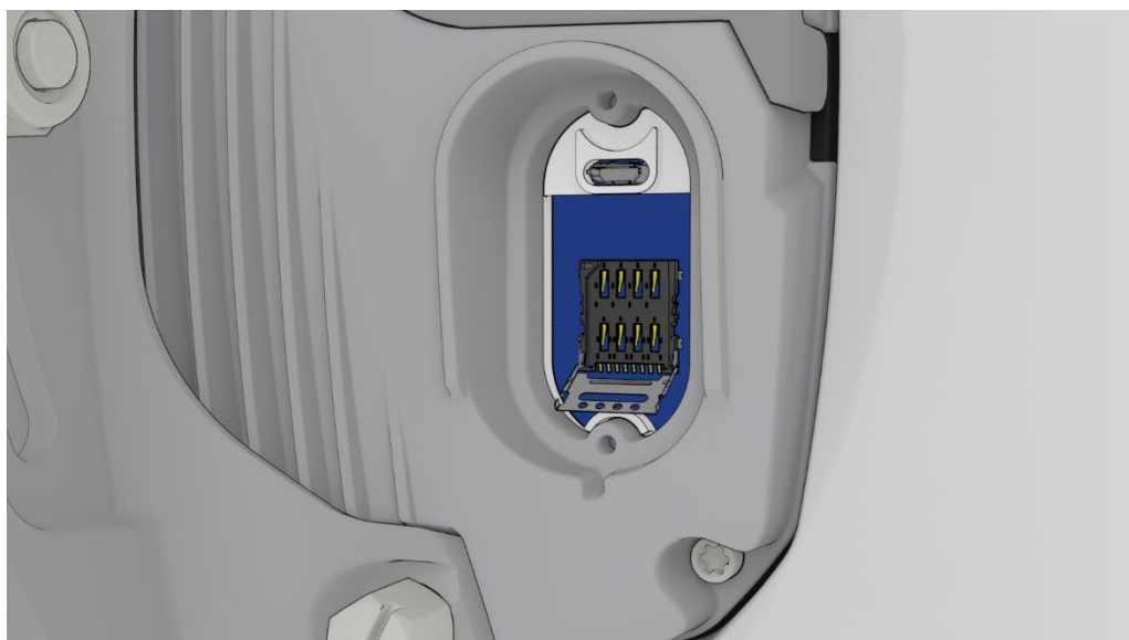
Figure 4 - Opening the SIM locking mechanism
