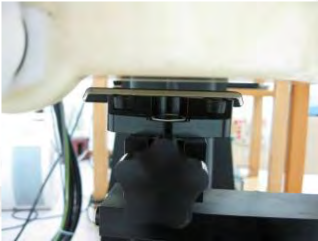
Fig.3 Front side of EUT is paralleled with flat phantom and spacing between EUT and Phantom is 10mm.
