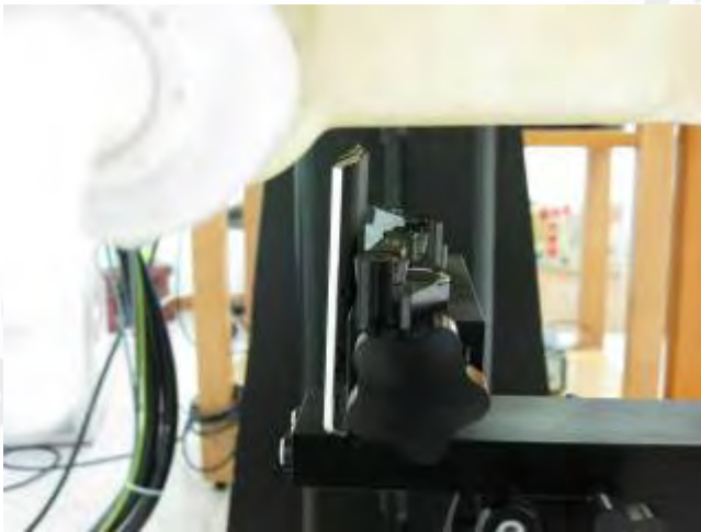
Fig.5 Top side of EUT is paralleled with flat phantom and spacing between EUT and Phantom is 10mm.
