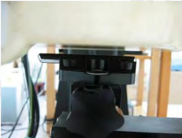
Fig.4 Back side of EUT is paralleled with flat phantom and spacing between EUT and Phantom is 10mm.
