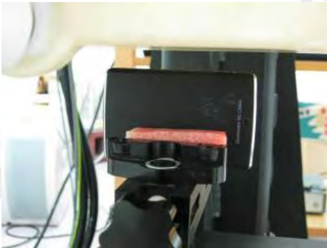
Fig.7 Left side of EUT is paralleled with flat phantom and spacing between EUT and Phantom is 10mm.
