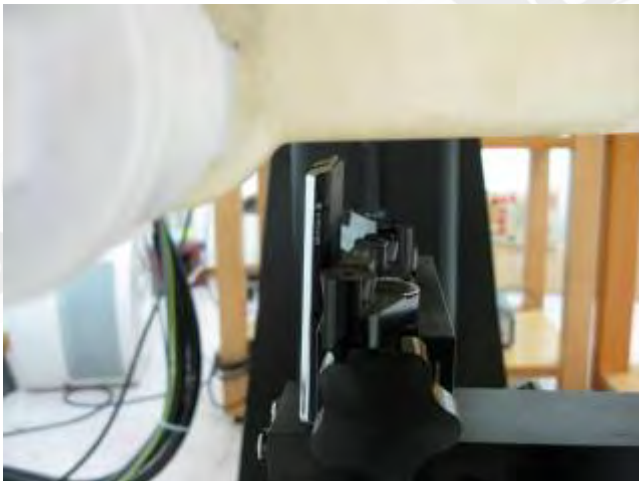
Fig.8 Bottom side of EUT is paralleled with flat phantom and spacing between EUT and Phantom is 10mm.
