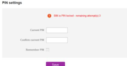
In the **Current PIN** field, enter the SIM PIN and then enter it again in the **Confirm current PIN** field. If you do not want to enter the PIN code each time the SIM is inserted, select the **Remember PIN** option. Click the **Save** button. The router displays “Success! The SIM unlock was successful”.
