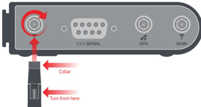
Please refer to the Device overview section for the antenna socket layout. If you have purchased a GPS antenna, remove the socket cap from the GPS antenna socket and attach the antenna to the socket in the same manner.
