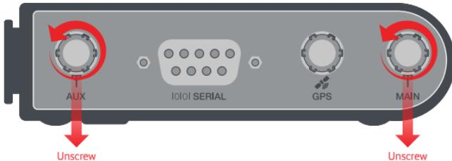
Then screw the antennas onto the sockets, turning them by the collar in a clockwise direction. When the collar has been sufficiently tightened, turn the antenna in a clockwise direction until it has reached the desired orientation.
