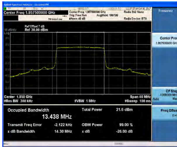
LTE Band 2 15MHz 16QAM CH-Middle
