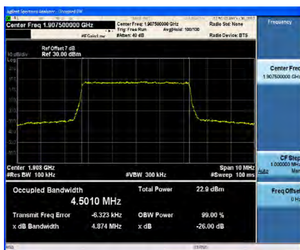
LTE Band 2 5MHz 16QAM CH-High
