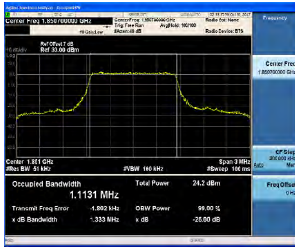
LTE Band 2 1.4MHz QPSK CH-Middle
