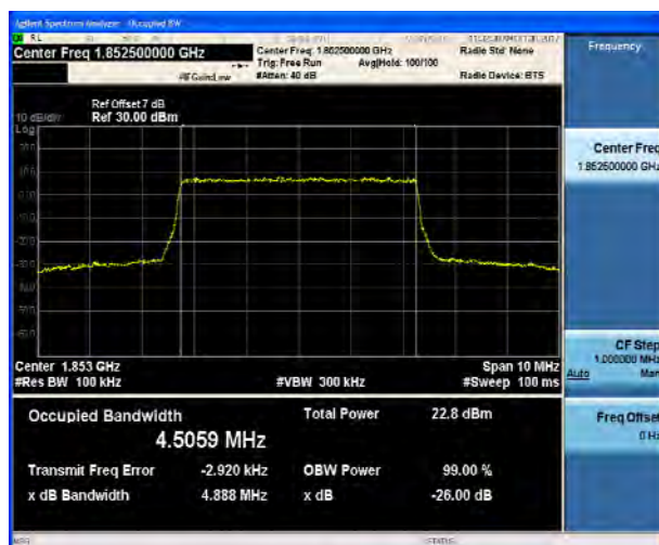
LTE Band 2 5MHz 16QAM CH-Middle
