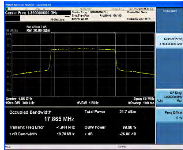
LTE Band 2 20MHz 16QAM CH-Middle
