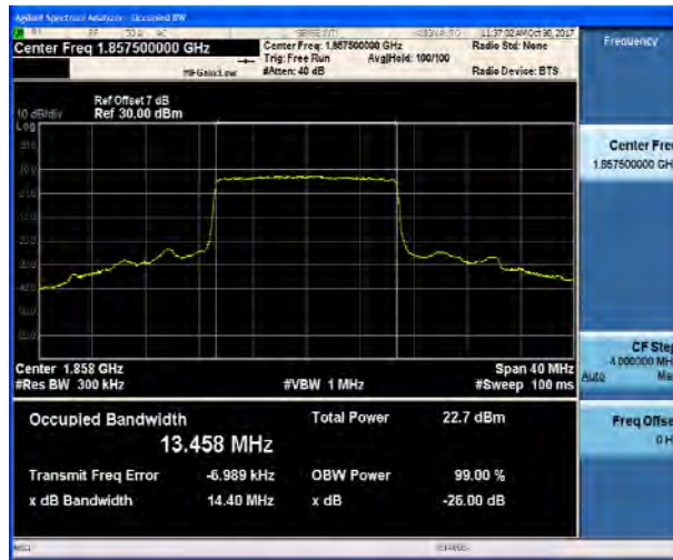
LTE Band 2 15MHz QPSK CH-Middle
