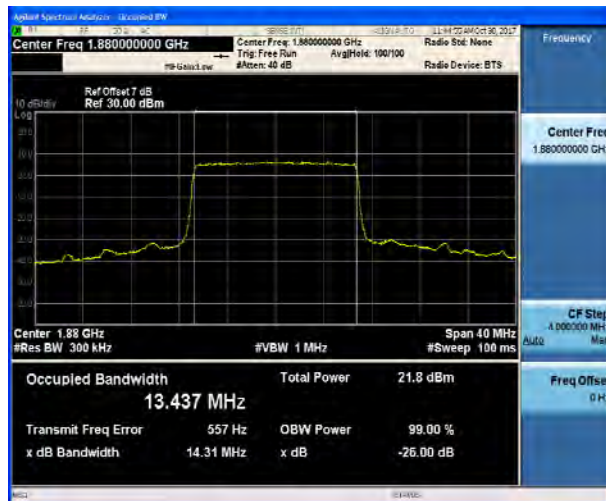
LTE Band 2 15MHz 16QAM CH-High
