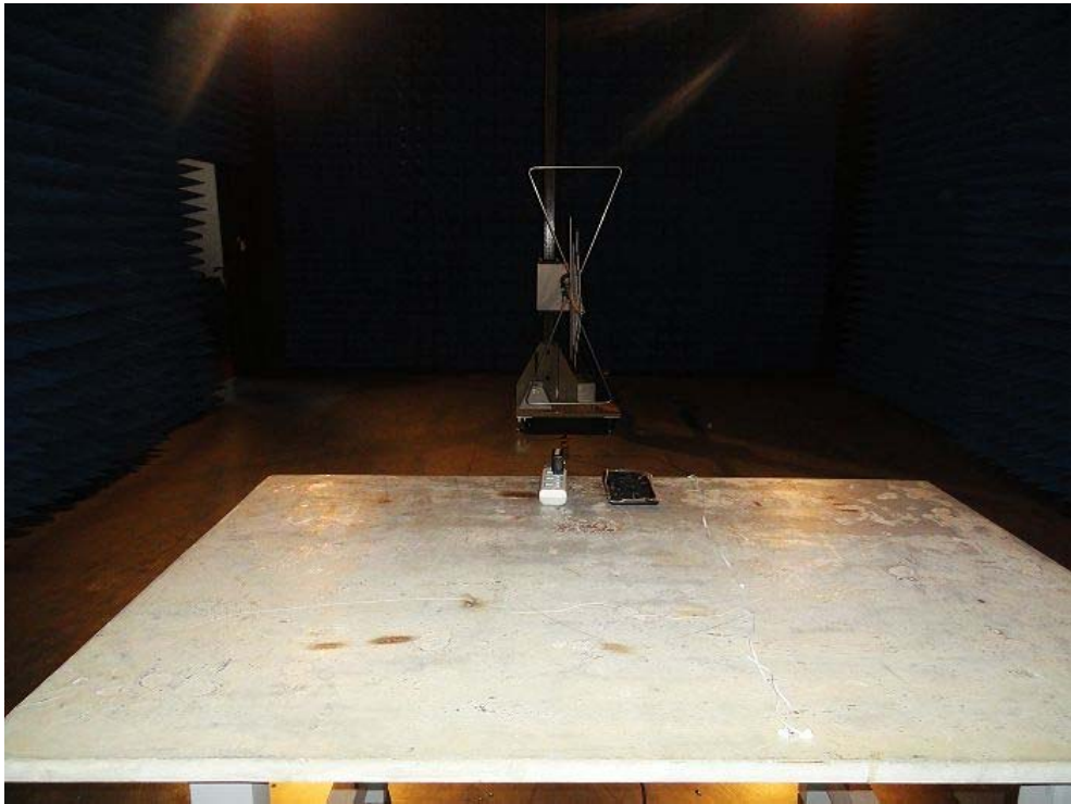
Radiated Emission Test Setup:
