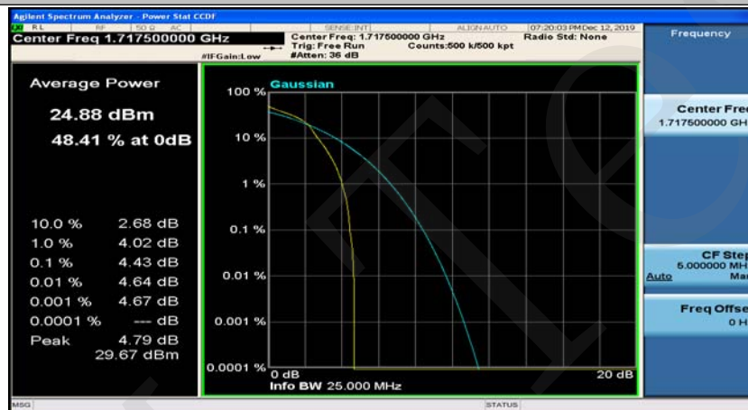
(Channel Bandwidth:15 MHz)_LCH_16QAM_1RB#74
