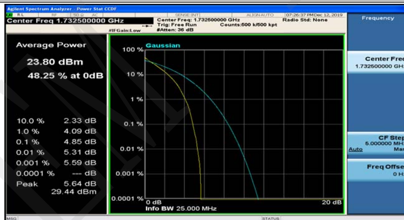
(Channel Bandwidth:20 MHz)_MCH_QPSK_50RB#50
