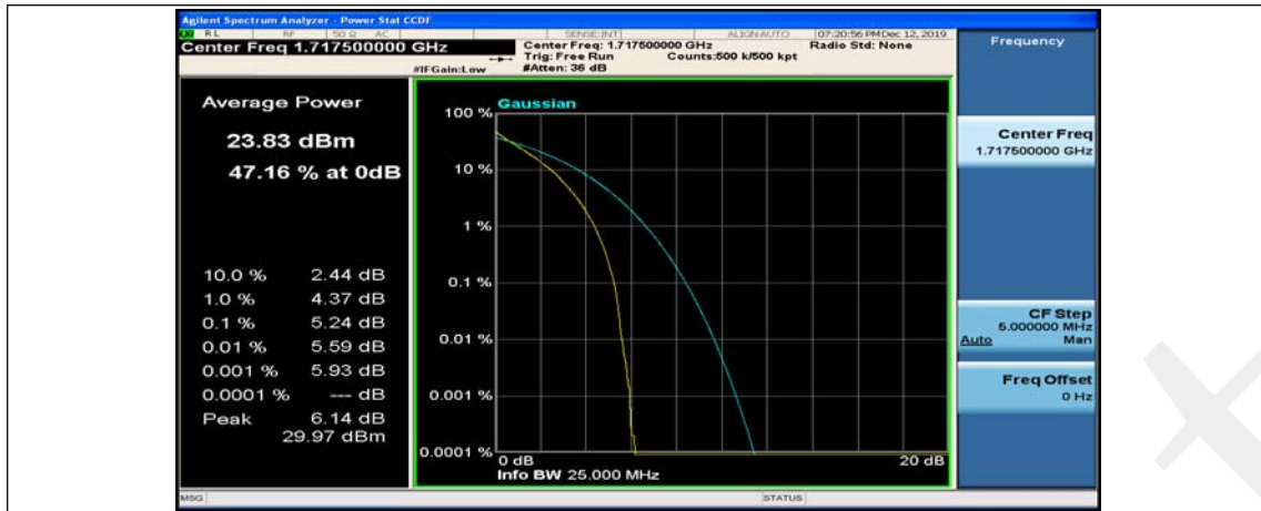
(Channel Bandwidth:15 MHz)_MCH_QPSK_1RB#0
