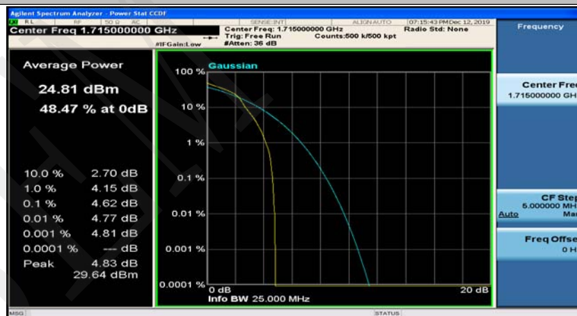
Channel Bandwidth: 10 MHz_LCH_16QAM_25RB#0
