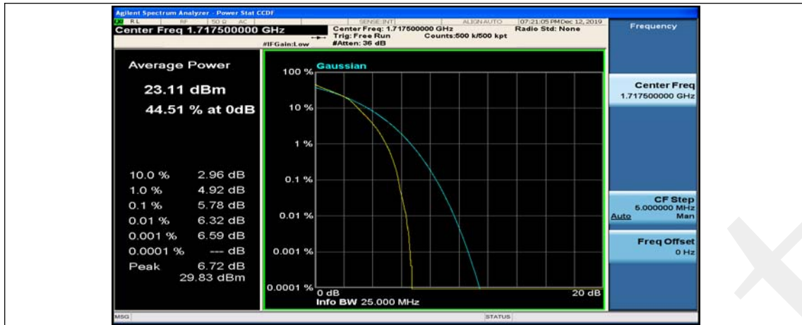
(Channel Bandwidth:15 MHz)_MCH_16QAM_1RB#0
