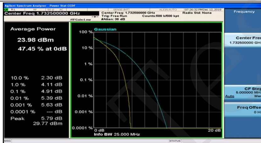
(Channel Bandwidth:20 MHz)_MCH_QPSK_50RB#25
