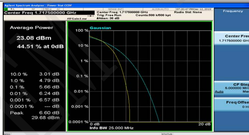
(Channel Bandwidth:15 MHz)_LCH_16QAM_75RB#0
