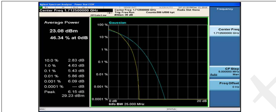
(Channel Bandwidth: 5 MHz)_MCH_16QAM_1RB#0
