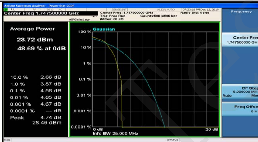
(Channel Bandwidth:15 MHz)_HCH_16QAM_37RB#0
