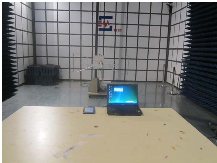
**Radiated Emission Test Setup (Above 1GHz)***Charging & Playing Mode*
