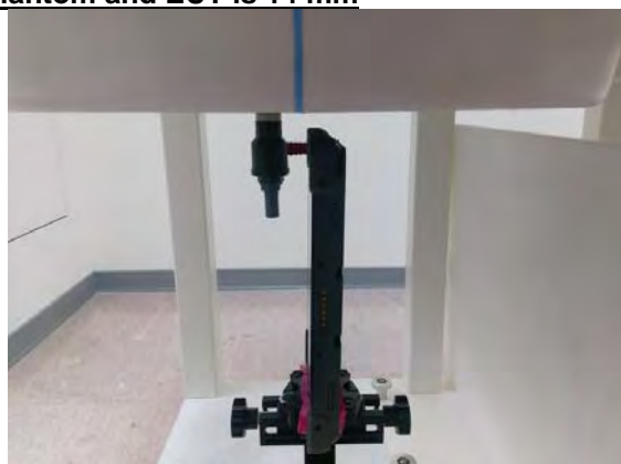
Fig.7 EUT Top side to flat phantom
