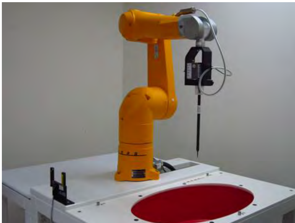
Fig.1 Photograph of the SAR measurement system
