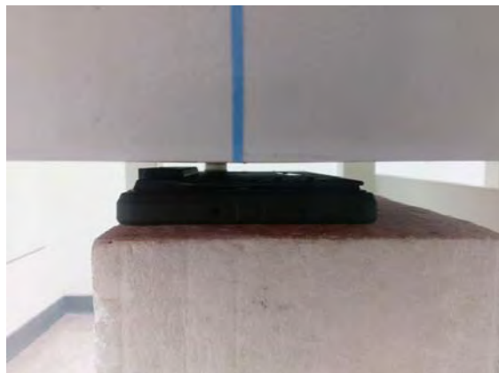
Fig.6 EUT back side to flat phantom
