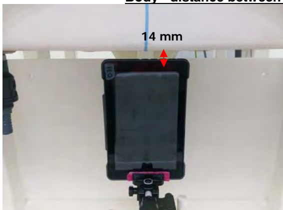
Fig.7 EUT Top side to flat phantom
