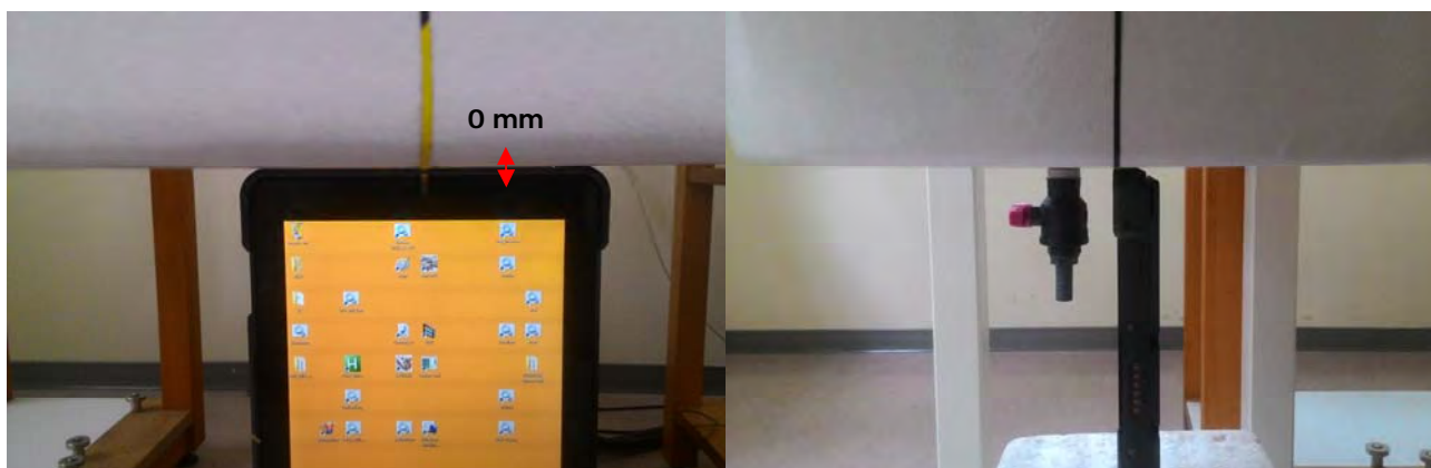
Fig.5 EUT Right side to flat phantom
