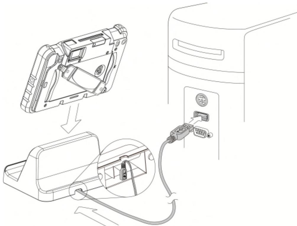
1. Connect the OTG USB cable to the connector on the bottom of the cradle charger and connect the other end to a PC to synchronize the two devices.
