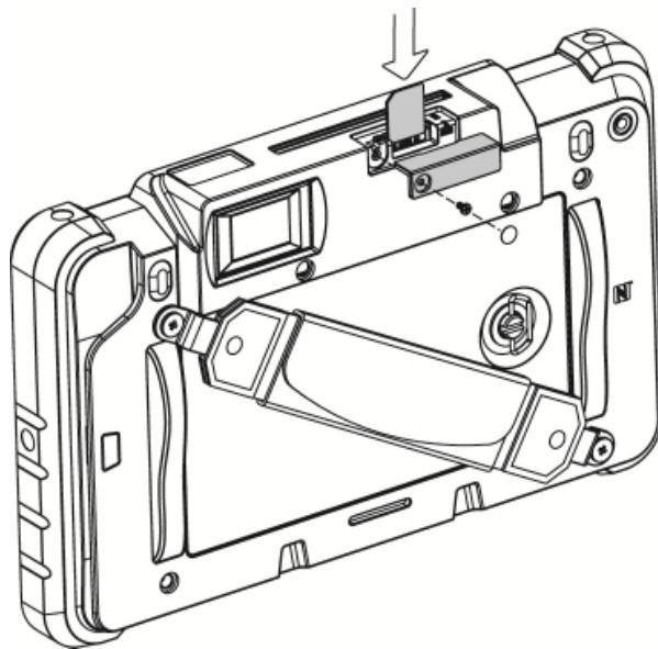
1. Loosen the screw(x1) to remove cover of 3G card slot.
