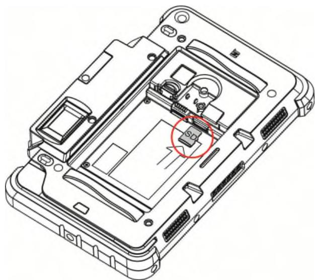
2. To install a Micro SD card insert the Micro SD card into slot until it snaps in place.
