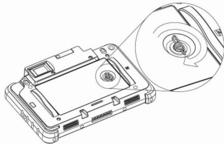
1. Loosen the pen screw counter-clockwise on the battery cover.
