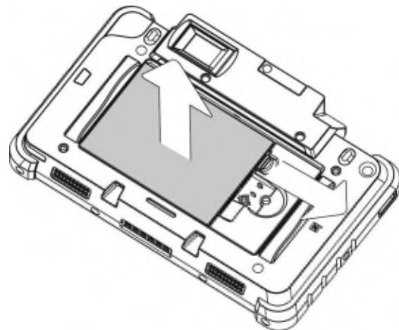
2. To remove the battery pull the plastic tab aside and gently lift the battery out of the system.
