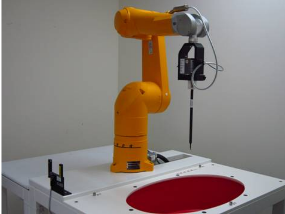
Fig.1 Photograph of the SAR measurement system
