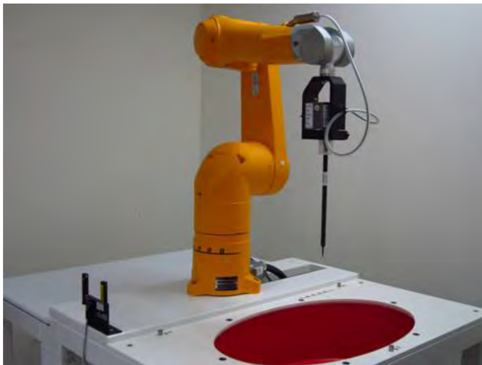
Fig.1 Photograph of the SAR measurement system
