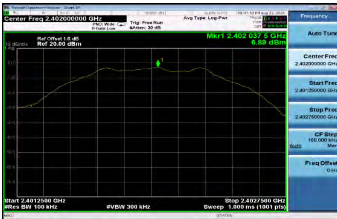
Power Spectral Density for Bandedge Limit (CH-High)
