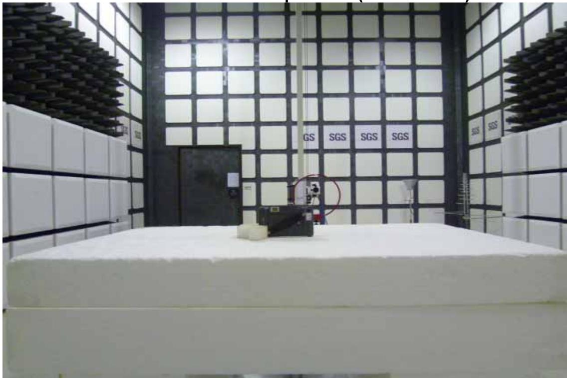
**Radiated Emission Setup Photos (Below 1GHz)**
