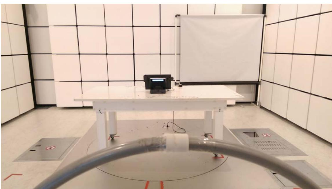
**Radiated emission test photos**
