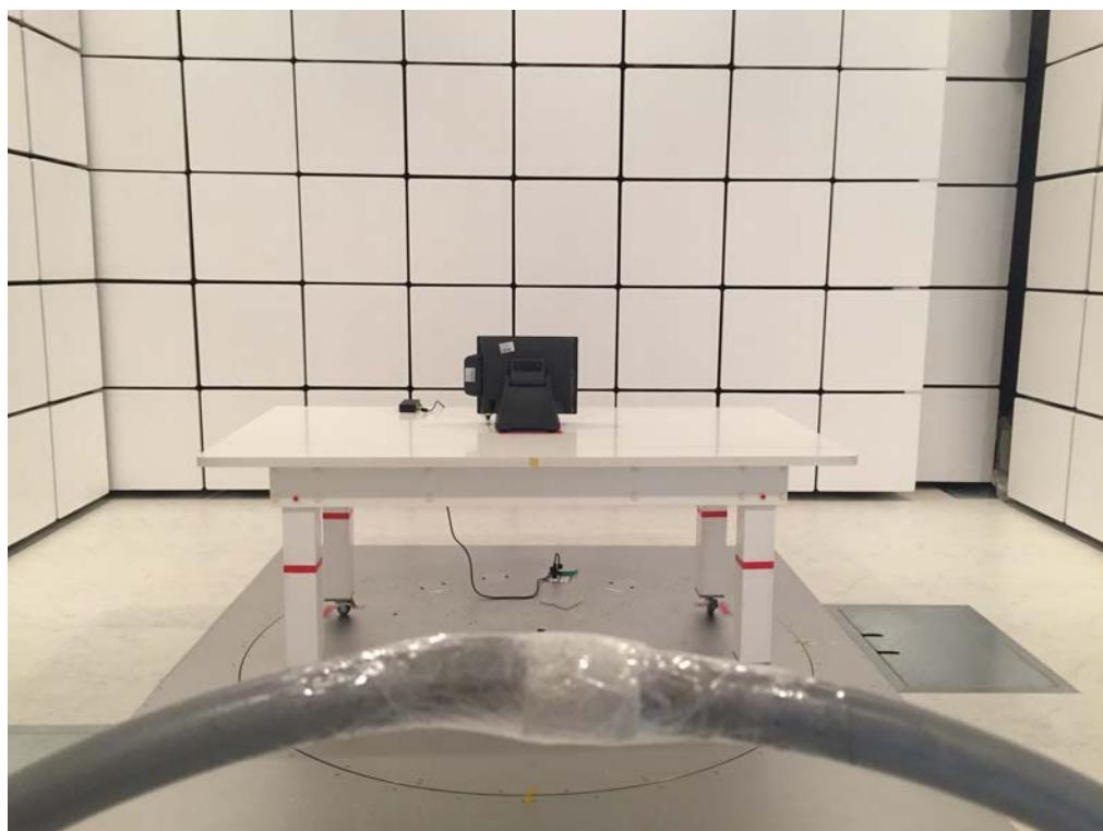
**Radiated emission test photos****30MHz to 1000MHz**
