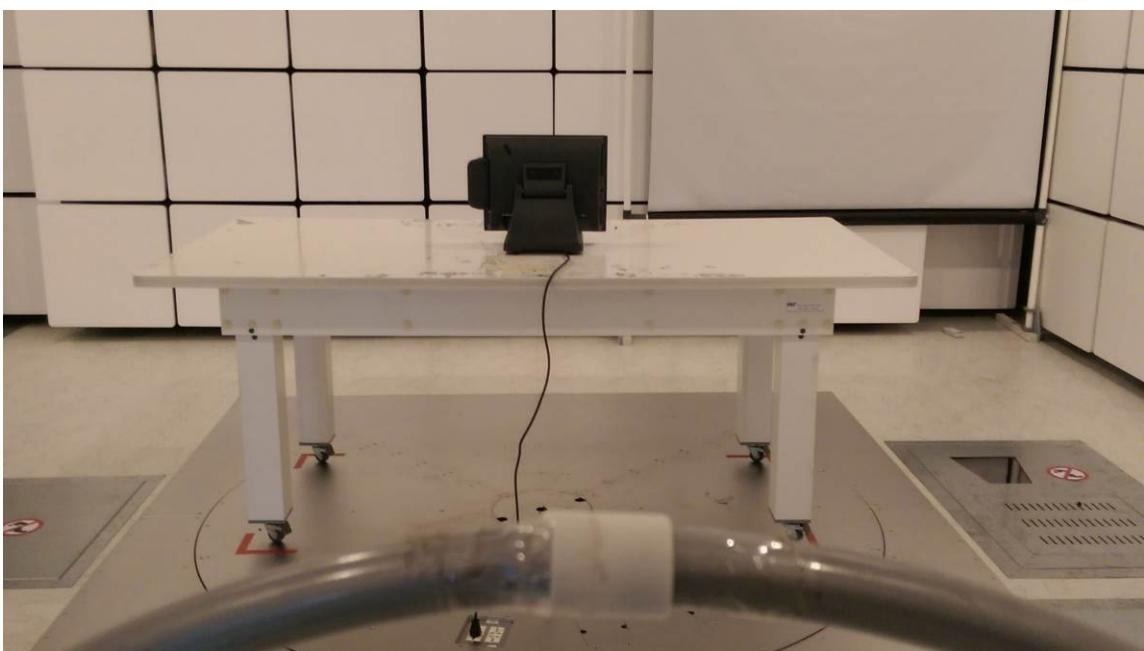
**Radiated emission test photos****30MHz to 1000MHz**
