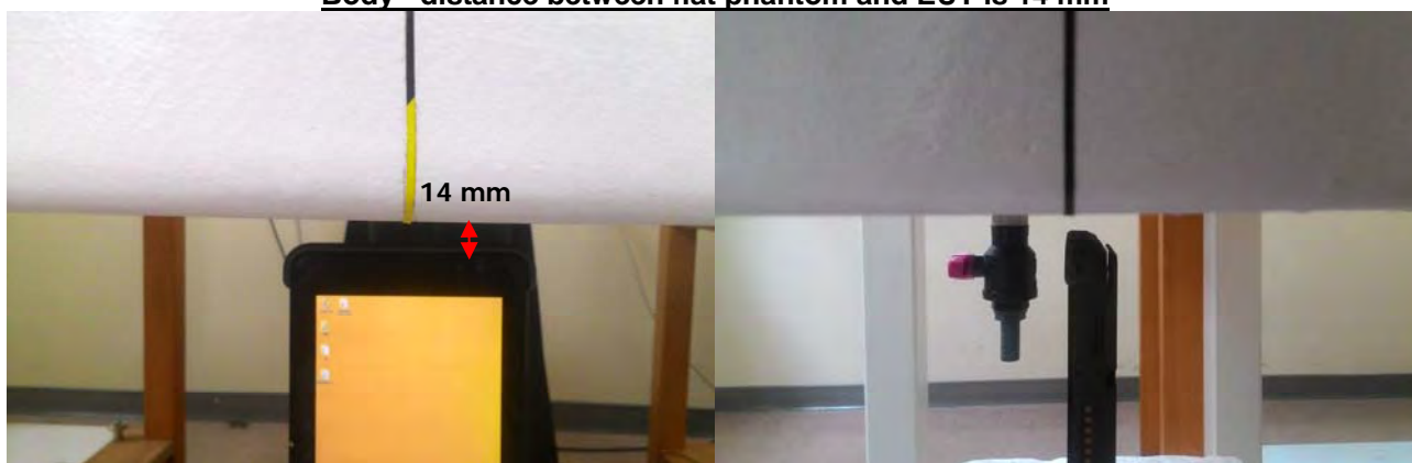
Fig.8 EUT Right side to flat phantom
