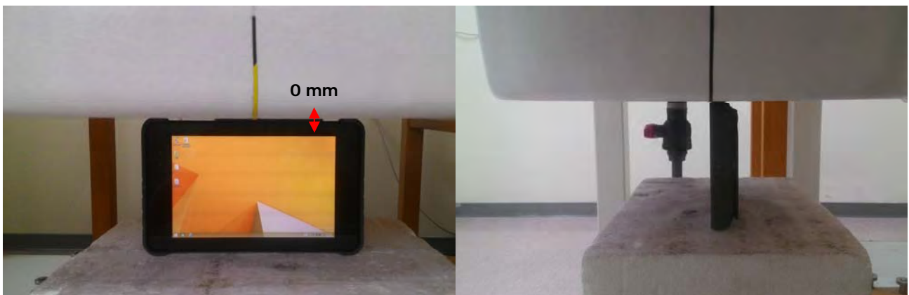
Fig.4 EUT Top side to flat phantom
