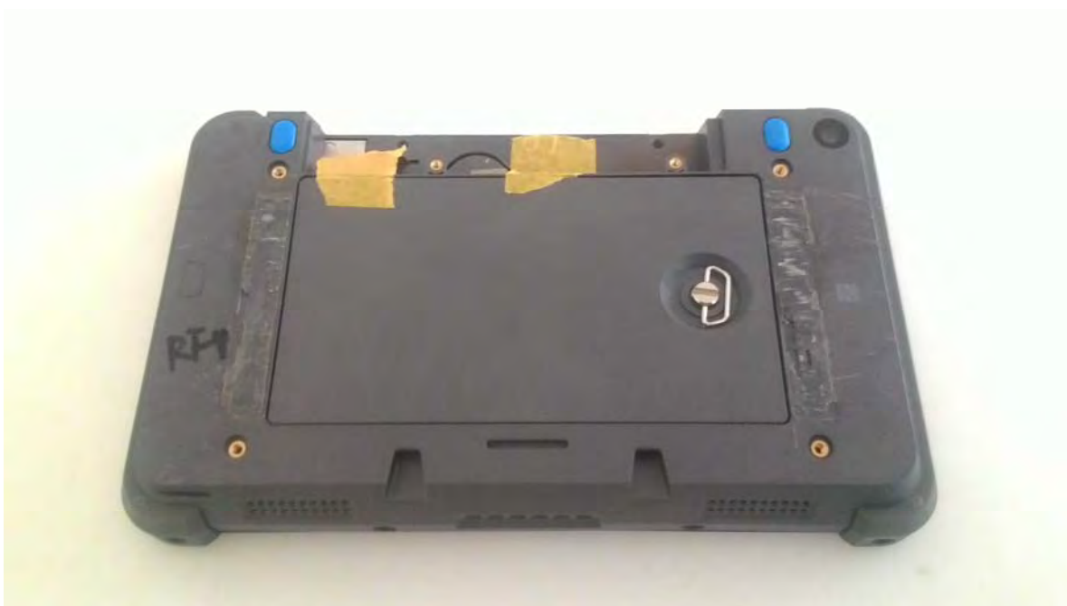
Fig.11 Back view of EUT (remove scanner and rails for SAR testing via KDB inquiry)
