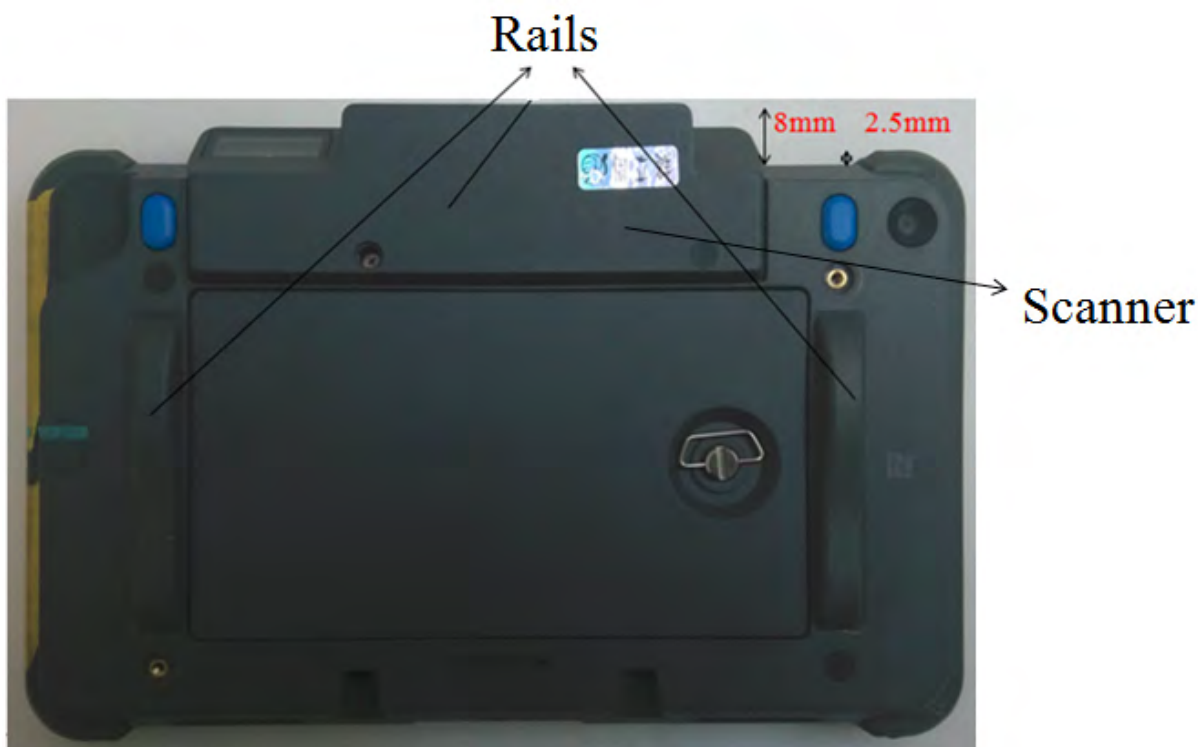
Fig.12 Back view of EUT(with scanner and rails)
