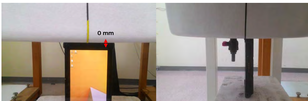
Fig.7 EUT Right side to flat phantom
