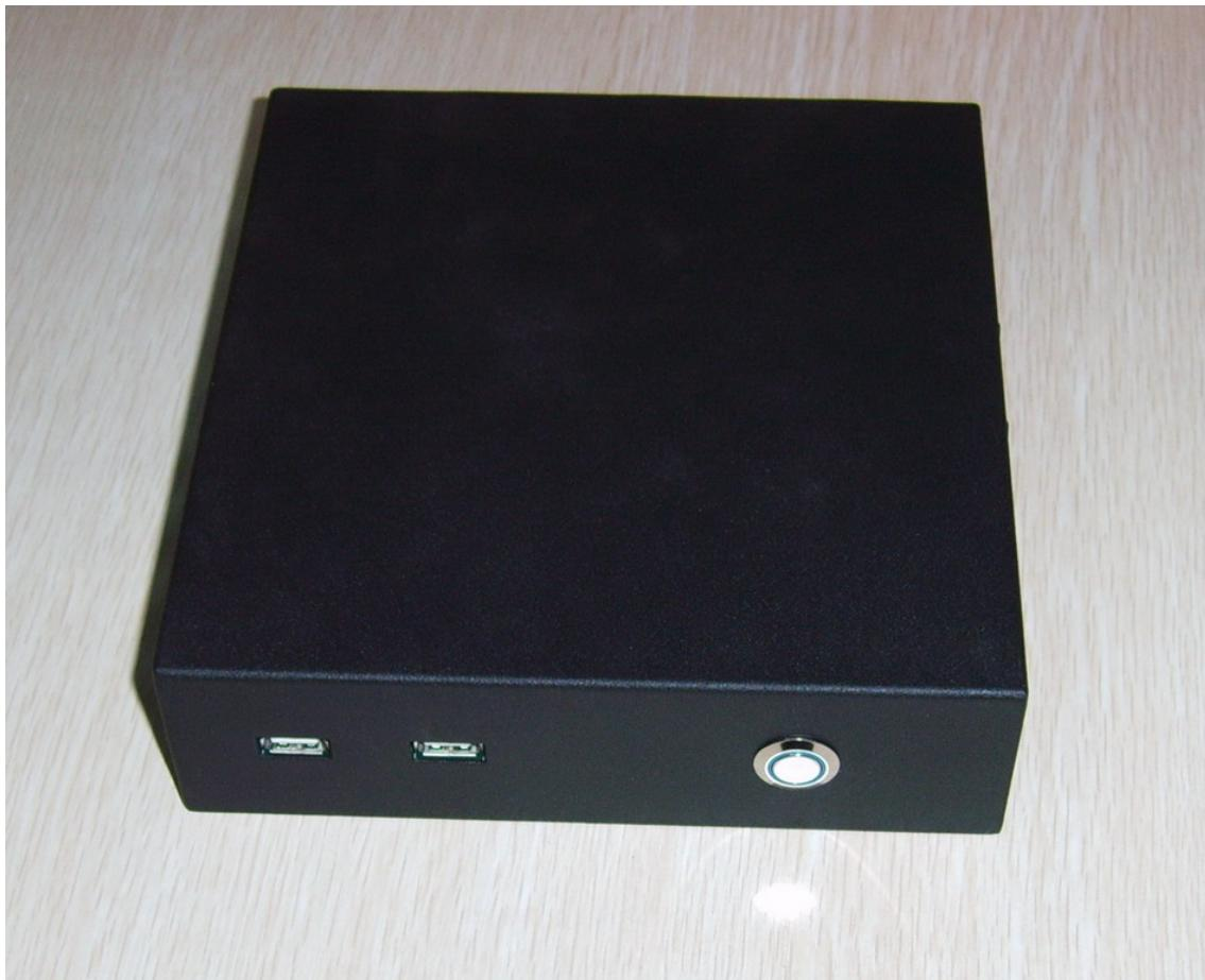
1. On the front panel there is a circular boot button, we can start the computer by pressing this button, and turn off the computer by pressing the boot button when the it is running. Around the circle button is the light which was used to indicate whether the computer is turned on
