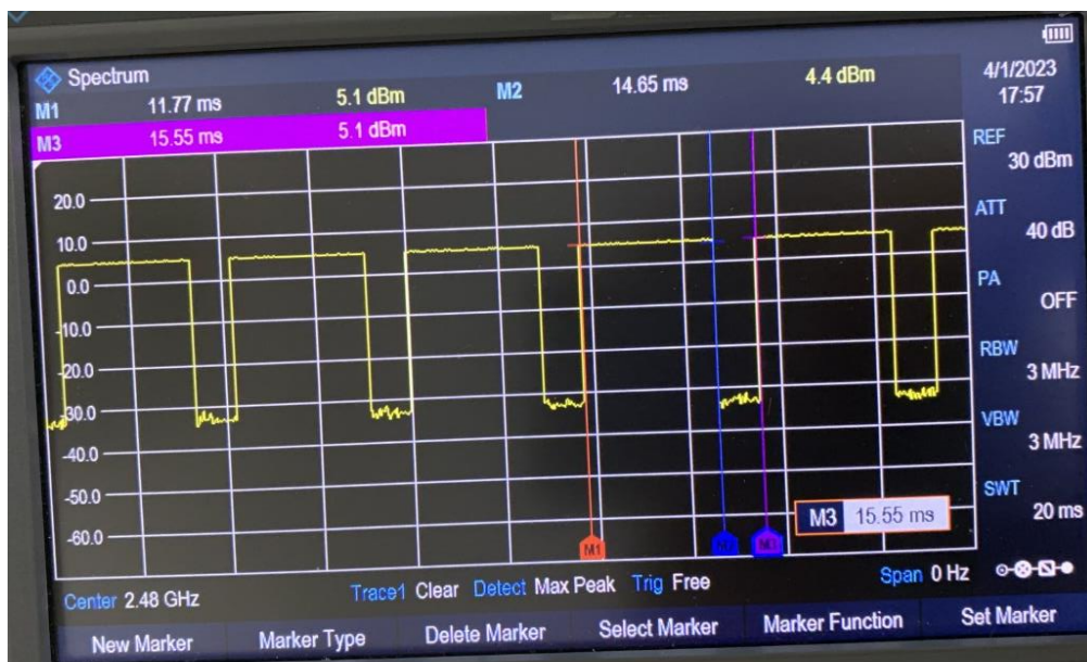
Time-domain plot for Bluetooth transmission signal
