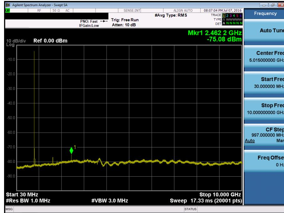
■ Secondary MODE (684 CH.) Conducted Spurious Emissions
