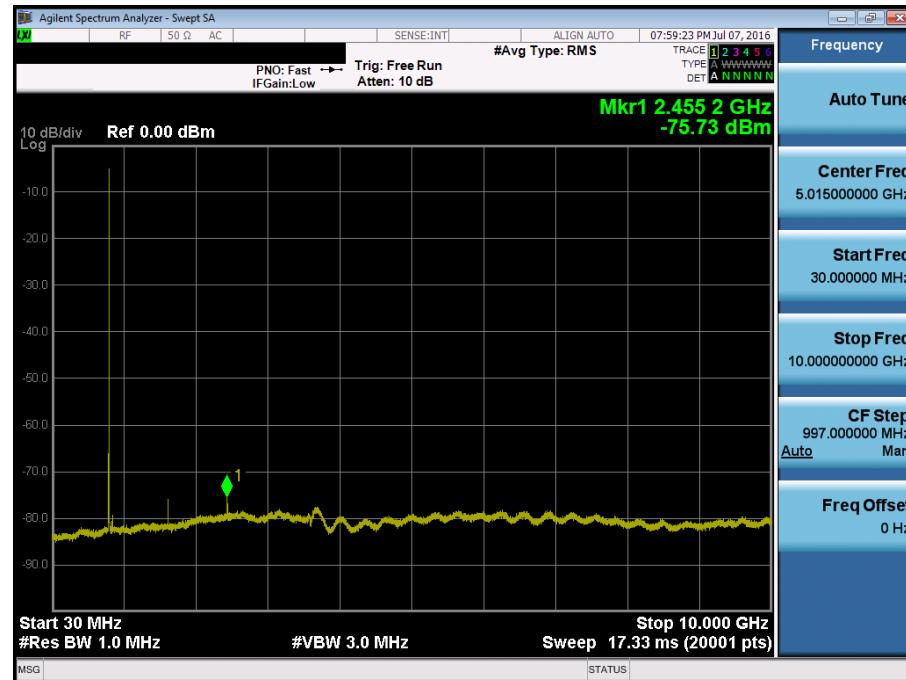
■ Secondary MODE (580 CH.) Conducted Spurious Emissions
