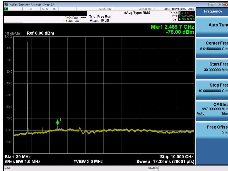
■ Secondary EVDO\_Rev.0 MODE (476 CH.) Conducted Spurious Emissions
