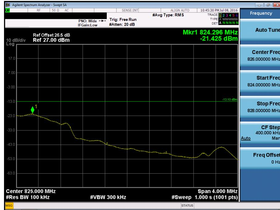
■ Secondary EVDO\_Rev.0 MODE (684 CH.) 4 MHz Span
