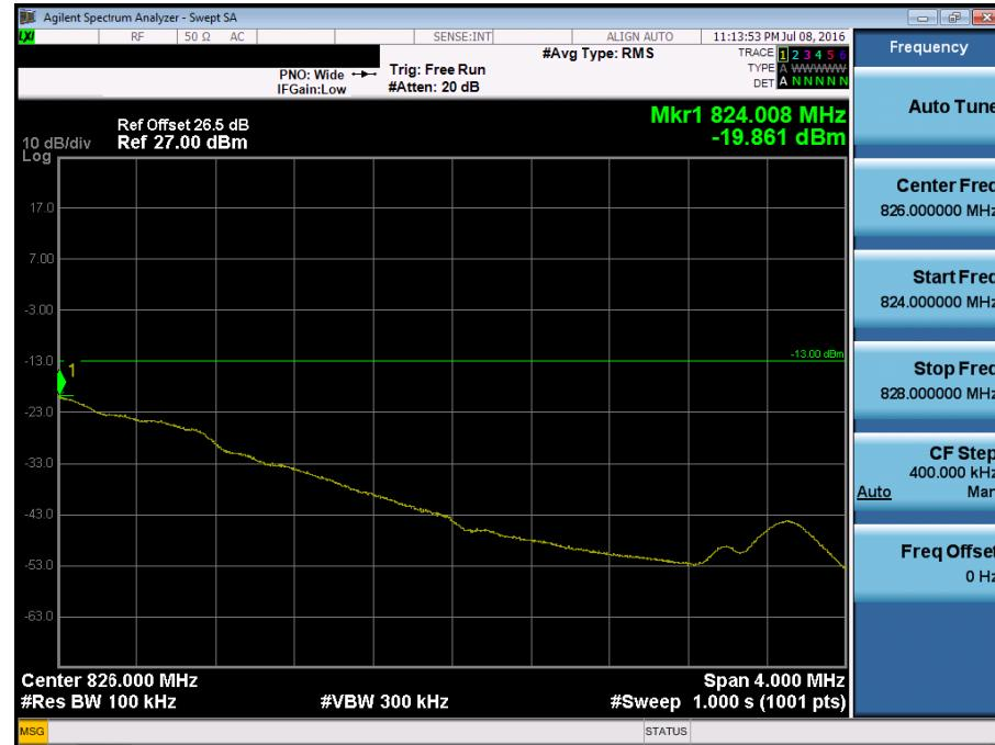
■ Secondary MODE (476 CH.) Conducted Spurious Emissions
