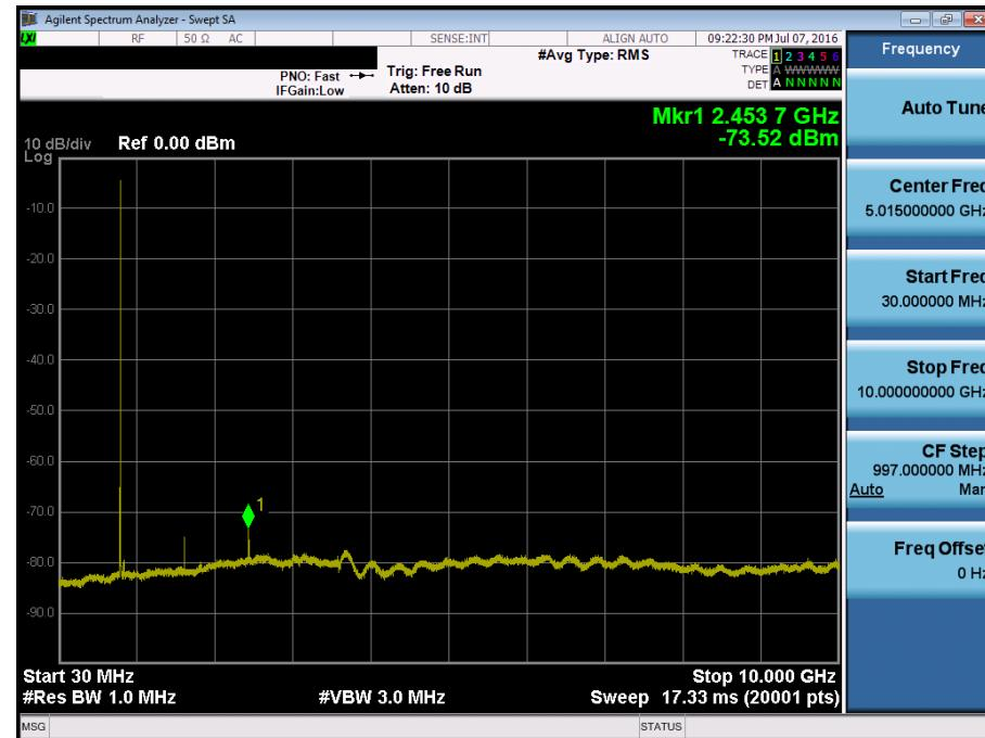
■ Secondary EVDO\_Rev.A MODE (580 CH.) Conducted Spurious Emissions
