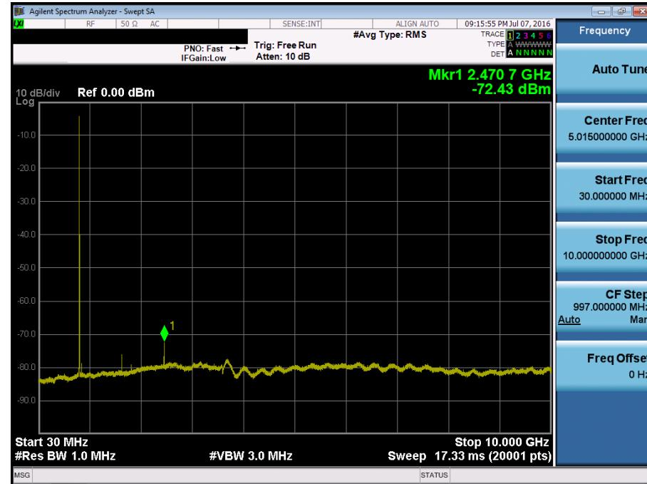
■ Secondary EVDO\_Rev.A MODE (476 CH.) Conducted Spurious Emissions
