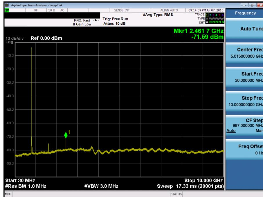
■ Secondary EVDO\_Rev.0 MODE (684 CH.) Conducted Spurious Emissions
