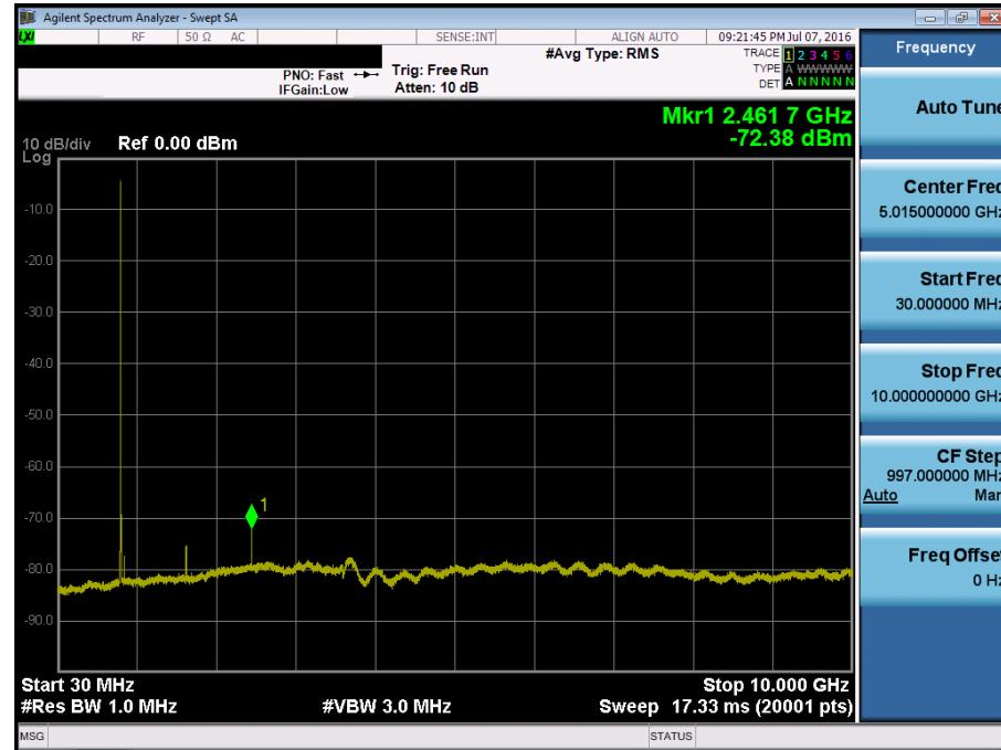
■ Secondary EVDO\_Rev.A MODE (684 CH.) Conducted Spurious Emissions
