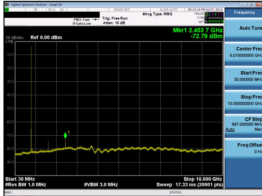
■ Secondary EVDO\_Rev.0 MODE (580 CH.) Conducted Spurious Emissions
