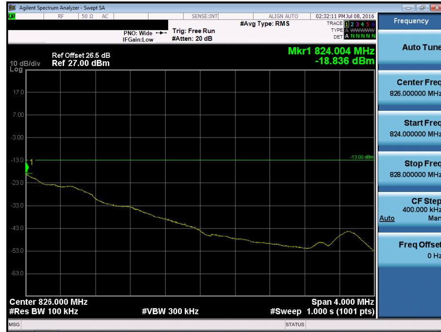
■ Secondary EVDO\_Rev.A MODE (684 CH.) 4 MHz Span
