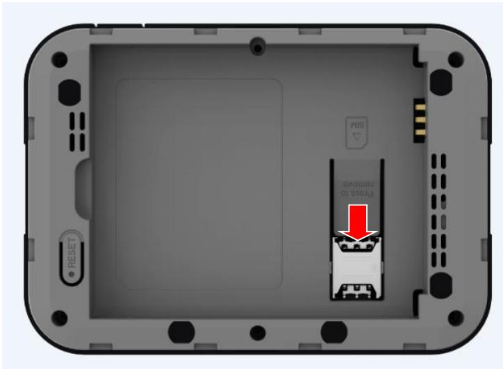
3. Remove the SIM card by gently pressing down and sliding outwards.
