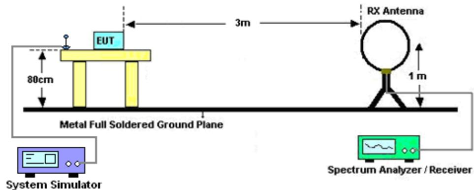
For radiated test from 30MHz to 1GHz
