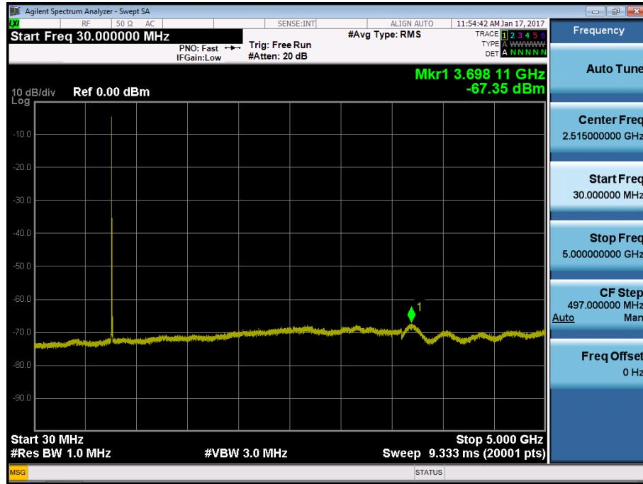
BAND 13. Conducted Spurious Plot\_2 (23255ch\_5MHz\_QPSK\_RB 1\_0)
