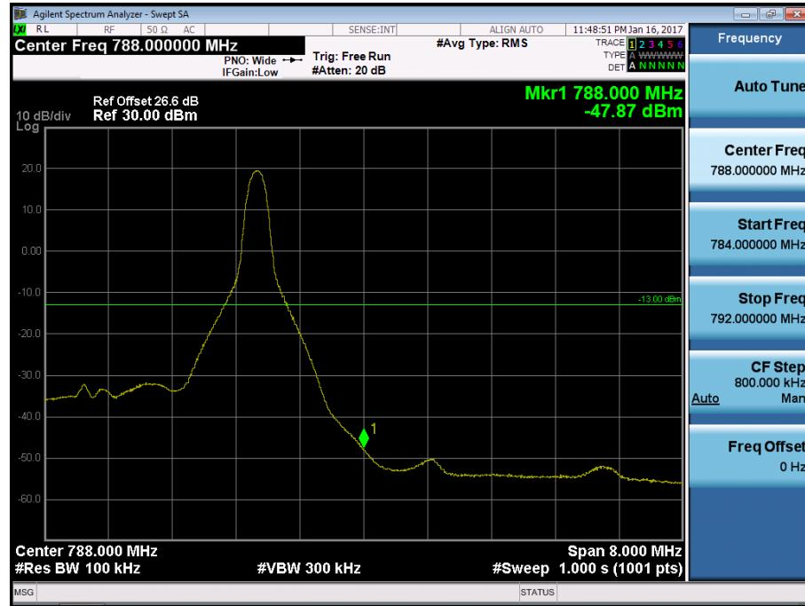
BAND 13. Lower & Upper Band Edge Plot (10M BW Ch.23230 QPSK RB 50)
