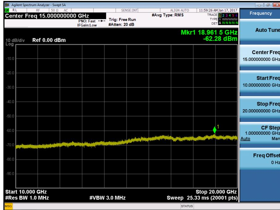
BAND 4. Conducted Spurious Plot\_1 (20175ch\_5MHz\_QPSK\_RB 1\_0)
