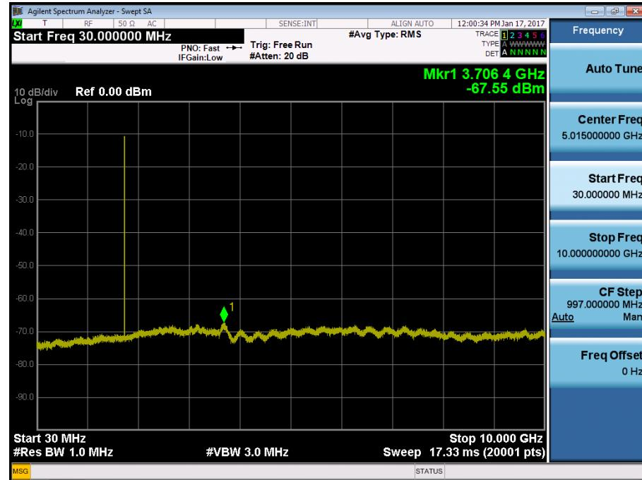
BAND 4. Conducted Spurious Plot\_2 (19975ch\_5MHz\_QPSK\_RB 1\_0)
