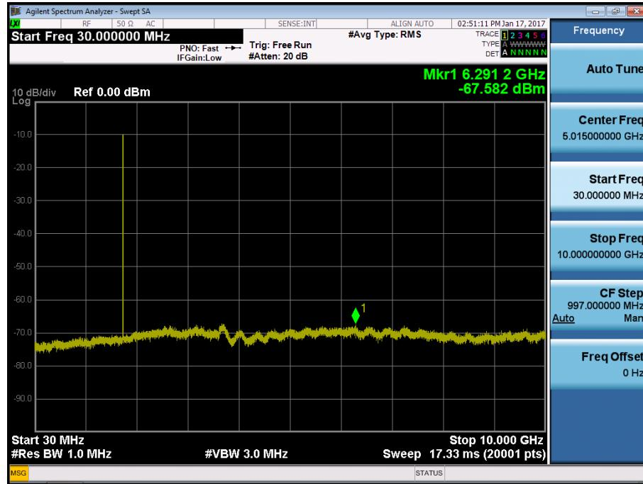
BAND 4. Conducted Spurious Plot\_2 (20375ch\_5MHz\_QPSK\_RB 1\_0)
