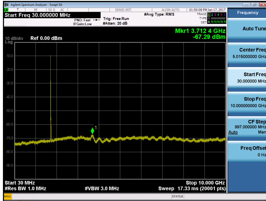
BAND 4. Conducted Spurious Plot\_2 (20300ch\_20MHz\_QPSK\_RB 1\_0)
