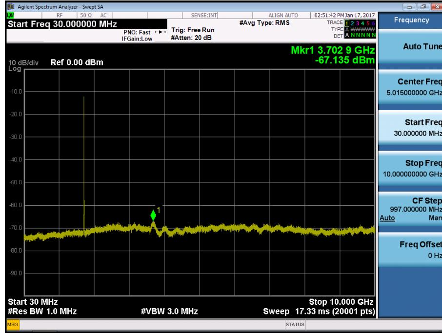
BAND 4. Conducted Spurious Plot\_2 (20175ch\_10MHz\_QPSK\_RB 1\_0)
