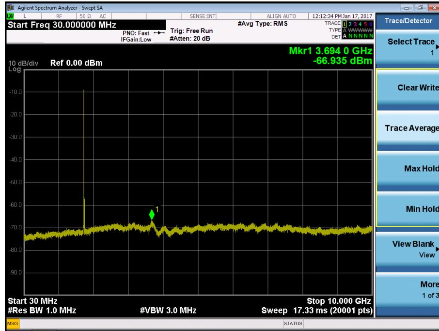
BAND 4. Conducted Spurious Plot\_2 (20325ch\_15MHz\_QPSK\_RB 1\_0)
