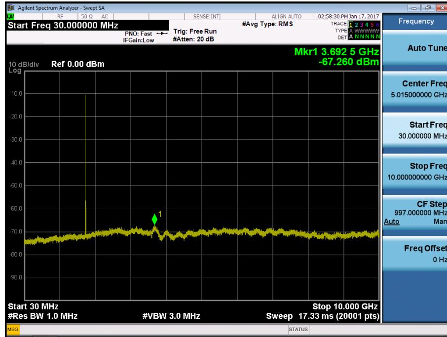
BAND 4. Conducted Spurious Plot\_2 (20350ch\_10MHz\_QPSK\_RB 1\_0)
