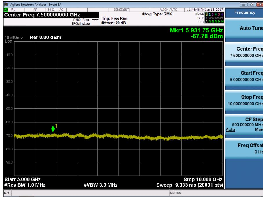
BAND 13. Conducted Spurious Plot\_1 (23230ch\_5MHz\_QPSK\_RB 1\_0)
