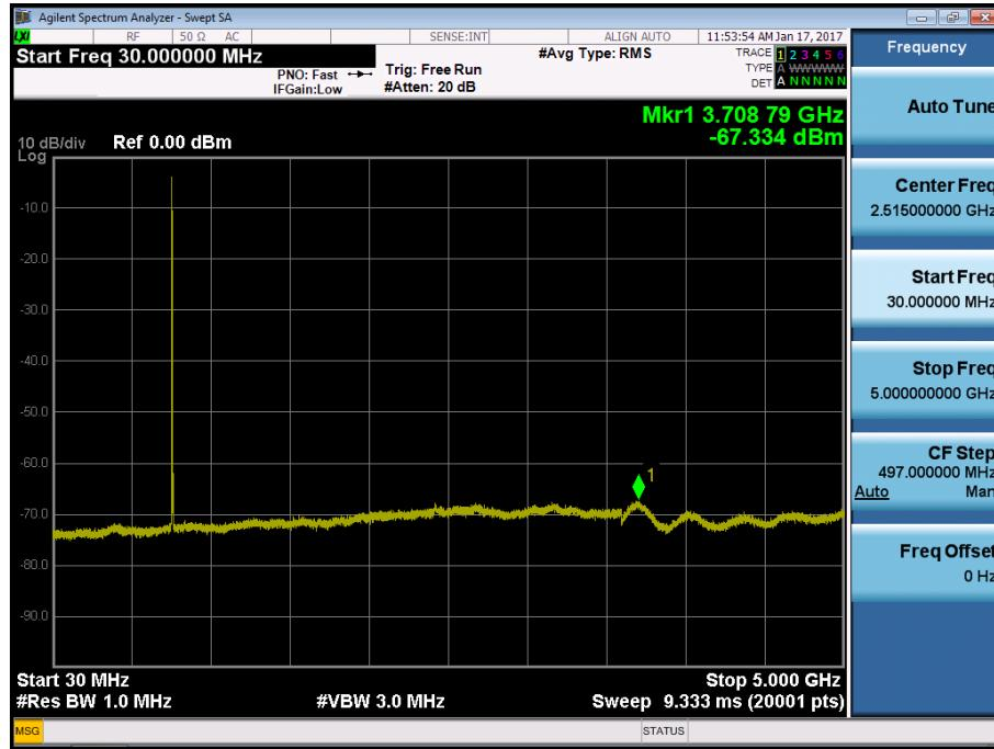
BAND 13. Conducted Spurious Plot\_2 (23205ch\_5MHz\_QPSK\_RB 1\_0)
