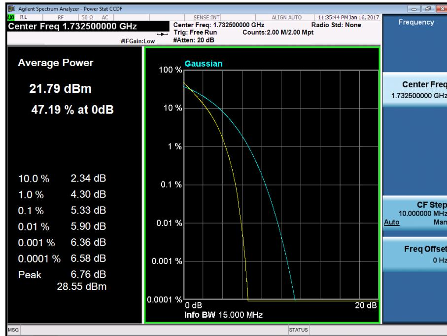
BAND 4. PAR Plot (15M BW\_Ch.20175\_16QAM\_RB75\_0)
