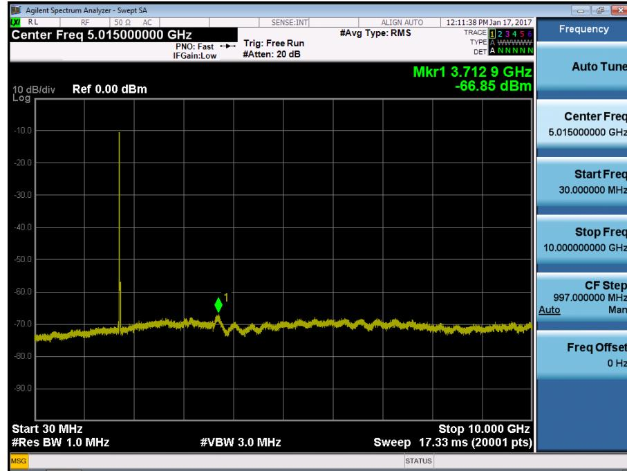
BAND 4. Conducted Spurious Plot\_2 (20175ch\_15MHz\_QPSK\_RB 1\_0)
