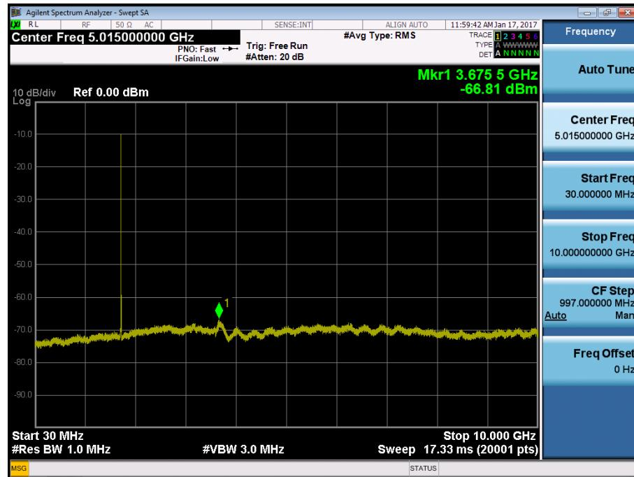
BAND 4. Conducted Spurious Plot\_2 (20175ch\_5MHz\_QPSK\_RB 1\_0)
