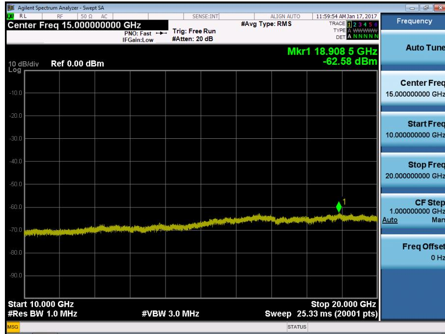
BAND 4. Conducted Spurious Plot\_1 (20375ch\_5MHz\_QPSK\_RB 1\_0)
