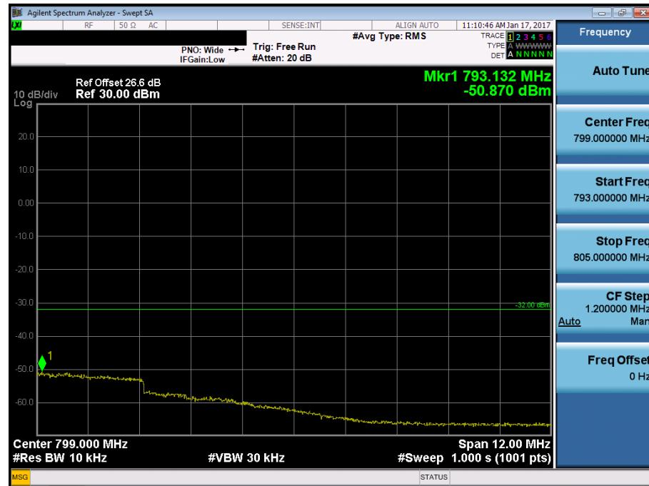
BAND 4. Conducted Spurious Plot\_1 (19975ch\_5MHz\_QPSK\_RB 1\_0)
