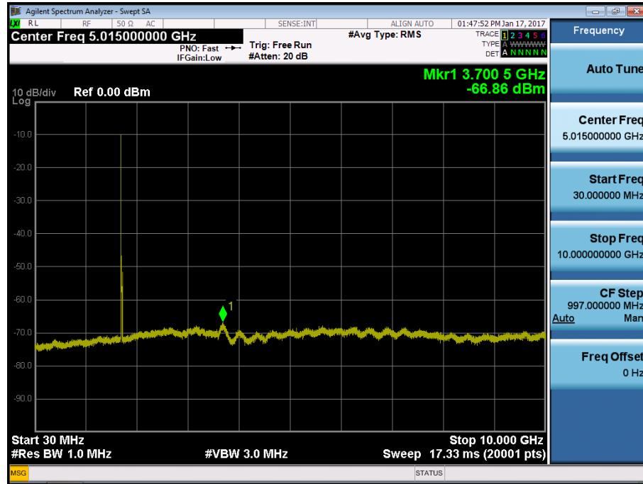
BAND 4. Conducted Spurious Plot\_2 (20050ch\_20MHz\_QPSK\_RB 1\_0)
