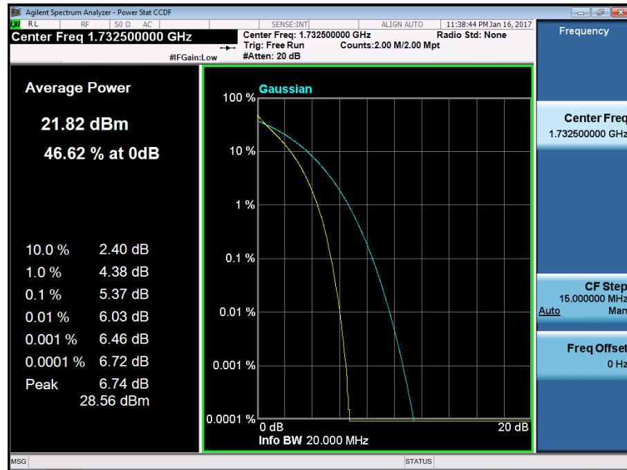
BAND 4. PAR Plot (20M BW\_Ch.20175\_16QAM\_RB100\_0)
