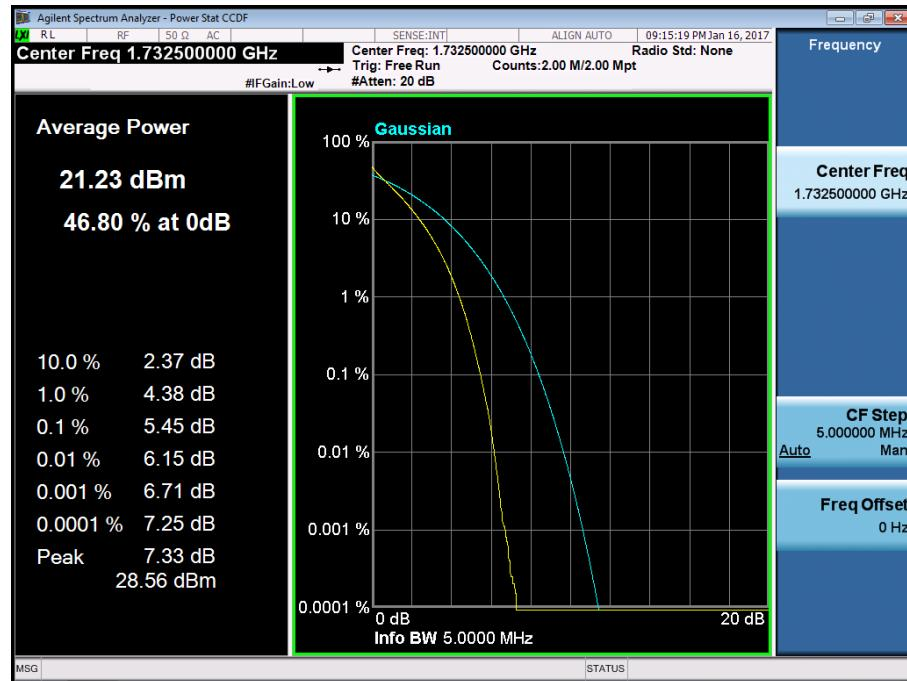
BAND 4. PAR Plot (5M BW\_Ch.20175\_16QAM\_RB25\_0)
