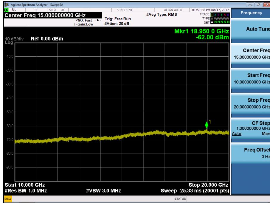
BAND 13. Conducted Spurious Plot\_1 (23205ch\_5MHz\_QPSK\_RB 1\_0)
