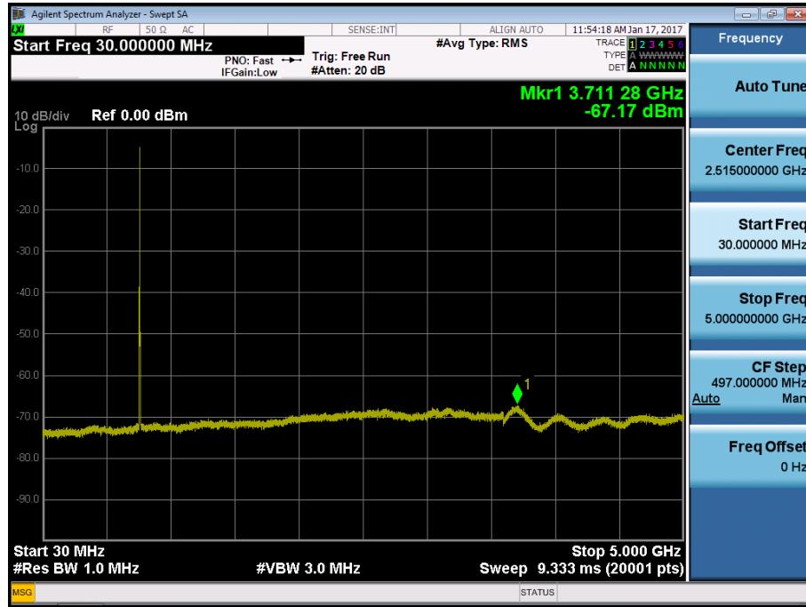
BAND 13. Conducted Spurious Plot\_2 (23230ch\_5MHz\_QPSK\_RB 1\_0)
