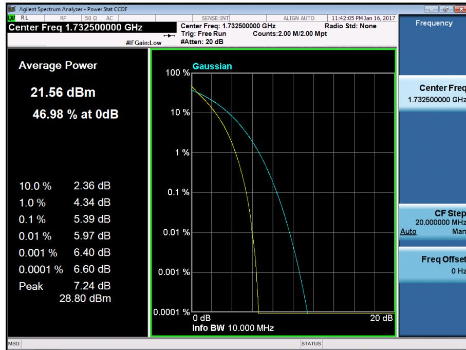
BAND 4. PAR Plot (10M BW\_Ch.20175\_16QAM\_RB50\_0)
