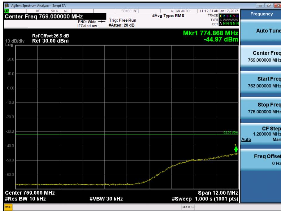
Band 13 Upper Band Edge Plot (10M BW Ch.23230 QPSK\_RB1\_Offset 24)
