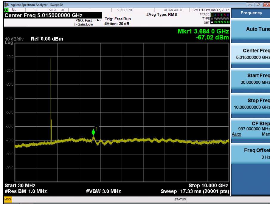
BAND 4. Conducted Spurious Plot\_2 (20025ch\_15MHz\_QPSK\_RB 1\_0)
