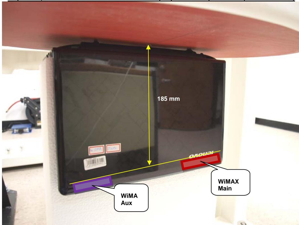
SAR Linearity test configuration w/ 2 mm from the Antenna-to-phantom (in direct contact to flat phantom)
