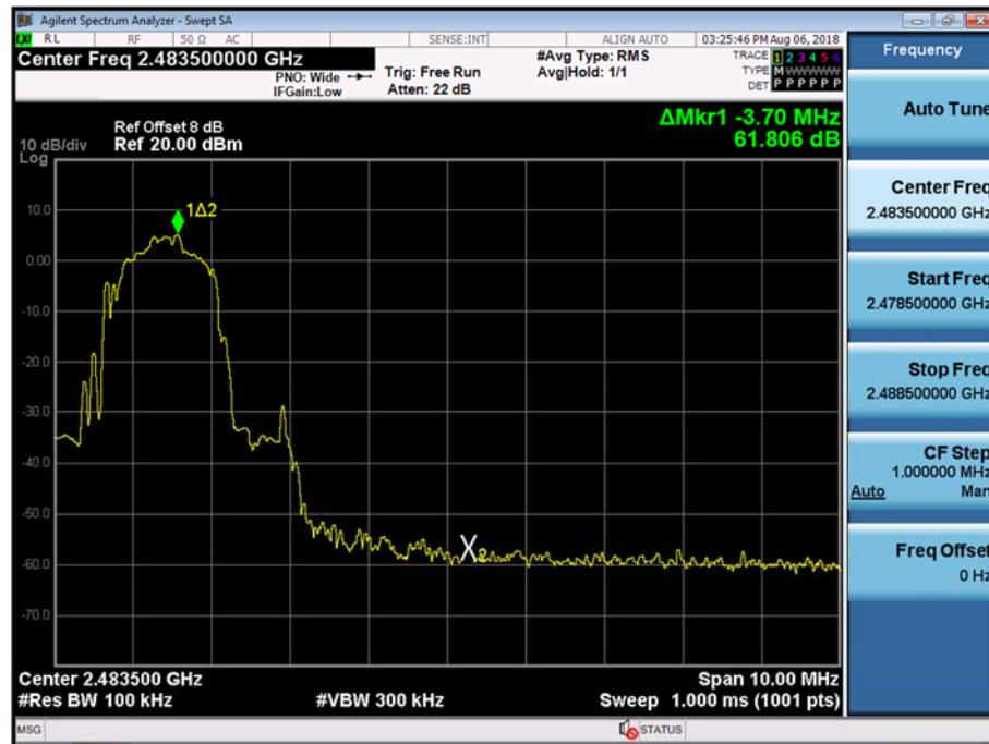
Test Plots with hopping (GFSK)
