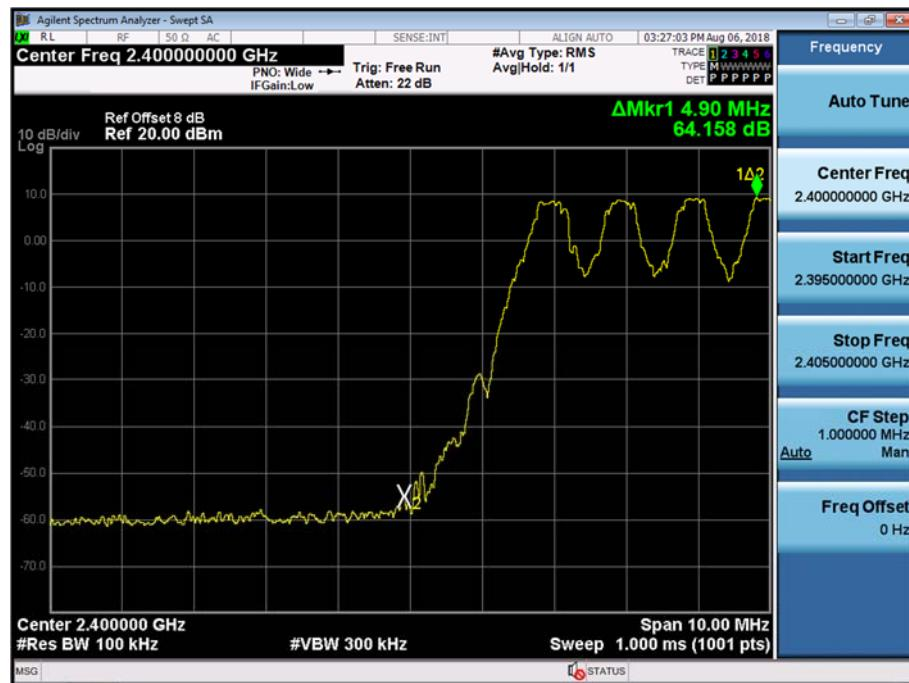
Test Plots with hopping (GFSK)
