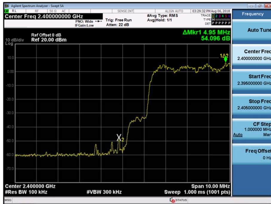
Test Plots with hopping (8DPSK)
