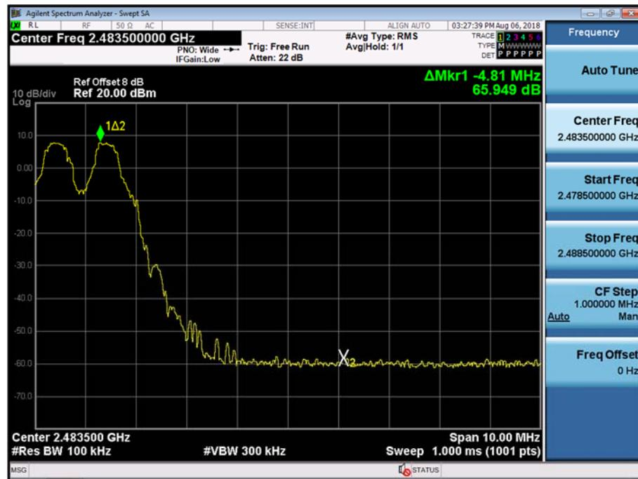
Test Plots with hopping (8DPSK)
