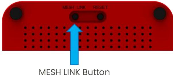
The Mesh LED pulse white until your Mesh controller will be successfully synced. This process time will take up to 6 minutes for syncing your Mesh controller.
