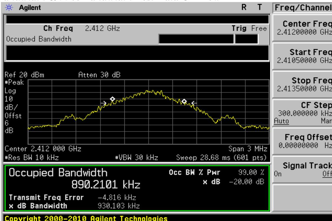
**20dB Bandwidth & 99% Bandwidth Test Data CH-Mid**
