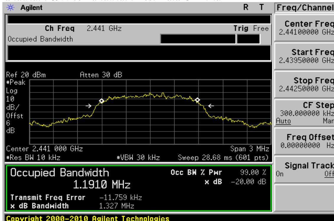
**20dB Bandwidth & 99% Bandwidth Test Data CH-High**
