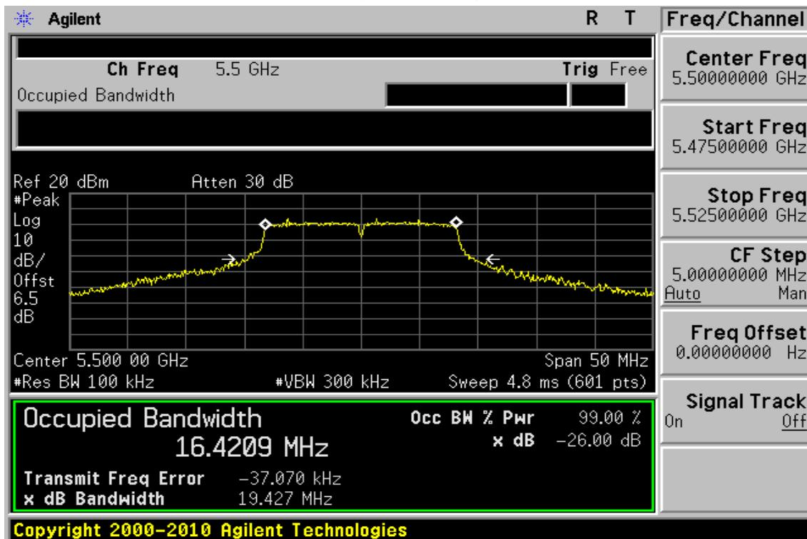
26dB Band Width Test Data CH-Mid (5580MHz)
