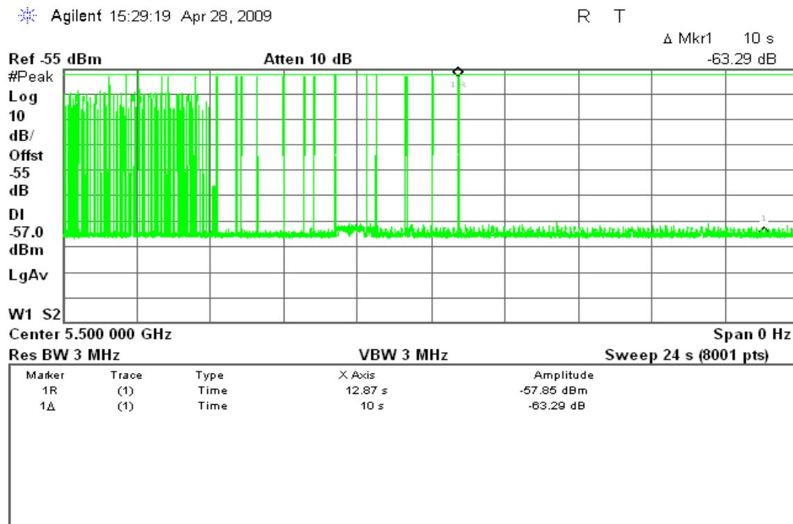
**draft 802.11n Wide-40 MHz Channel mode****Type 5 Channel Move Time Results**
