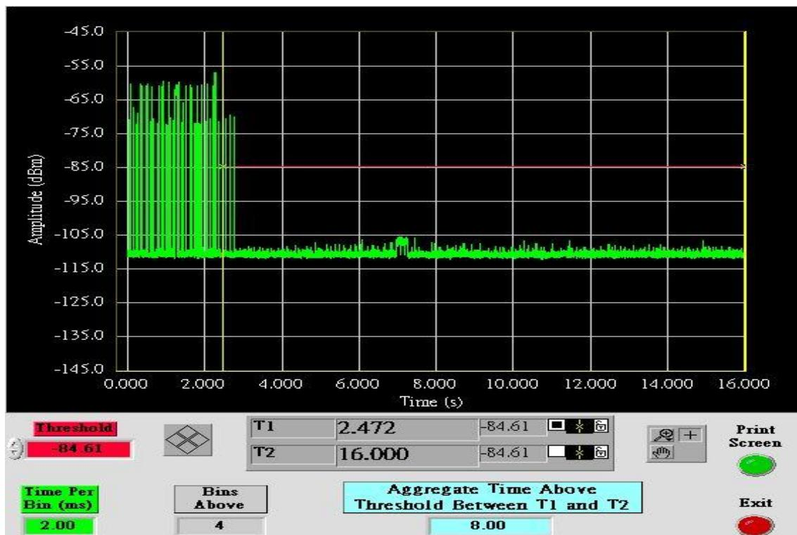
**draft 802.11n Standard-20 MHz Channel mode****Type 5 Channel Move Time Results**
