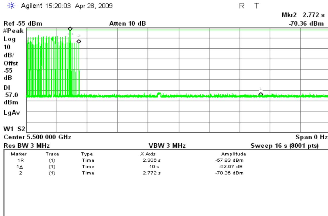
**draft 802.11n Wide-40 MHz Channel mode****Type 1 Channel Move Time Results***No non-compliance noted.*
