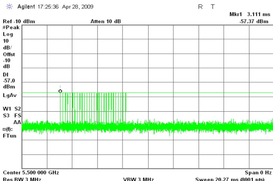
**Sample of Short Pulse Radar Type 3**
