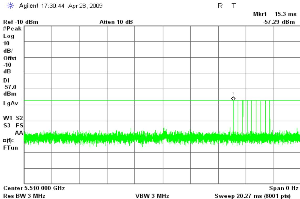
**Plot of WLAN Traffic from Slave**
