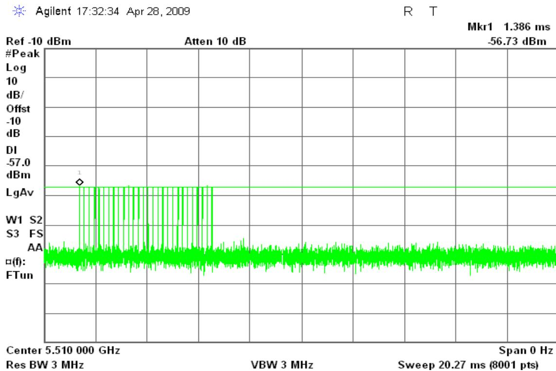
**Sample of Short Pulse Radar Type 3**
