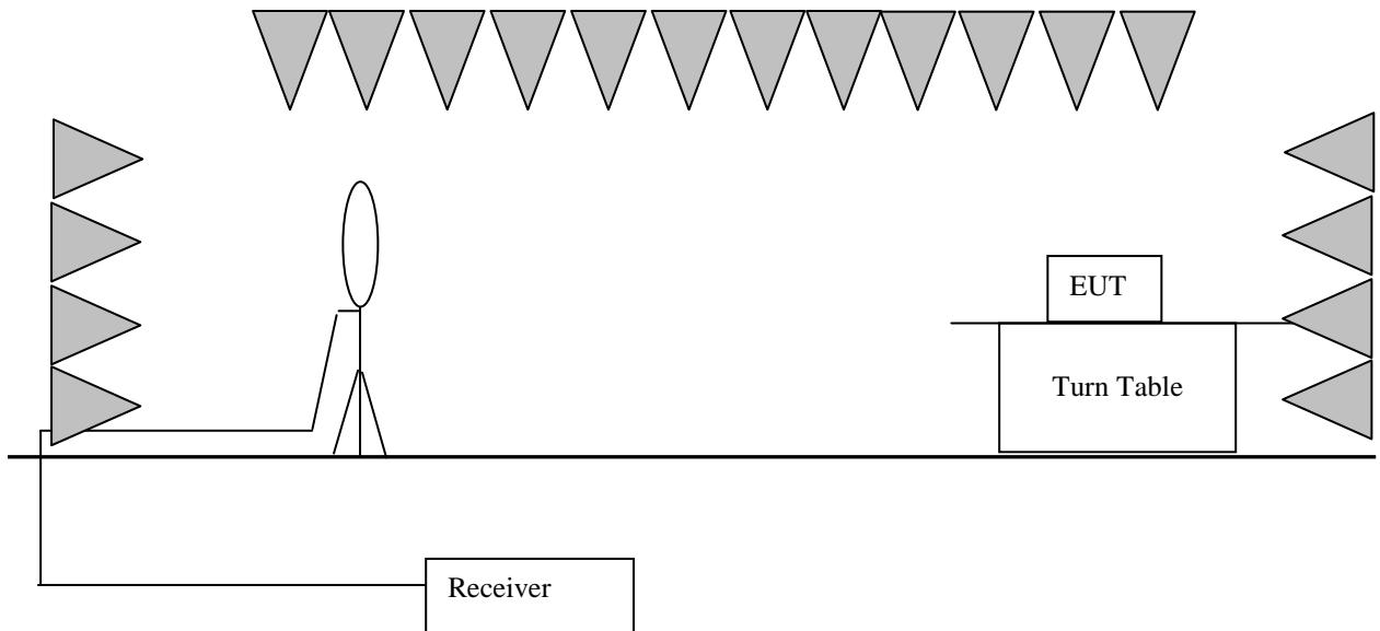
2) 30 MHz to 1 GHz emissions:
