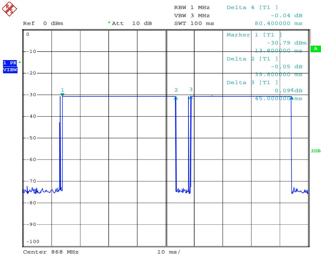
**1) Fundamental emission:****Antenna polarization: Horizontal:**
