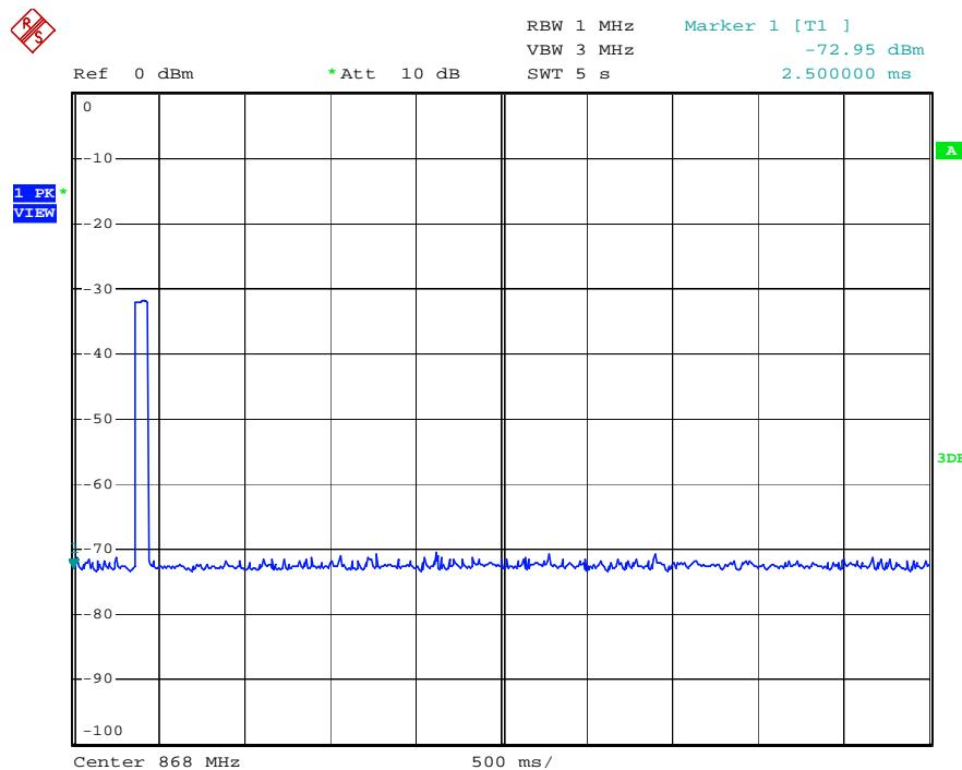
**3. Regulation 15.231 (a2)** A transmitter activated automatically shall cease transmission within 5 seconds after activation.
