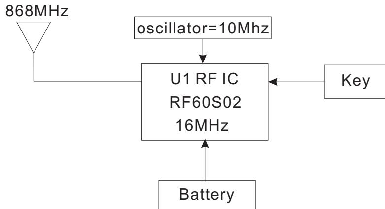
RF60 is the IC combines MCU AND RF together, LPOSC has a frequency of 24MHz, in order to lower down the power consumption we lower this number down to 16MHz in actual product
