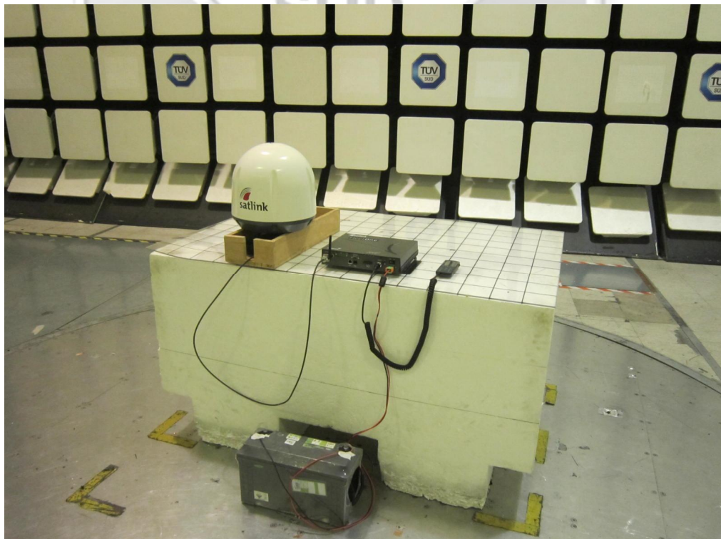
Radiated Emissions Test Setup (Rear View)
