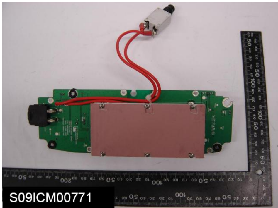
PCB views "Power Supply Board" of Fleet Broadband Satellite Communication System
