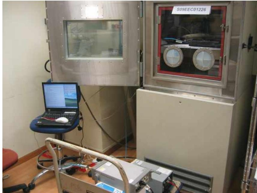
**Frequency Stability (Temperature Variation) Test Setup**
