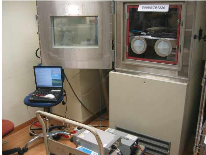
**Frequency Stability (Voltage Variation) Test Setup**
